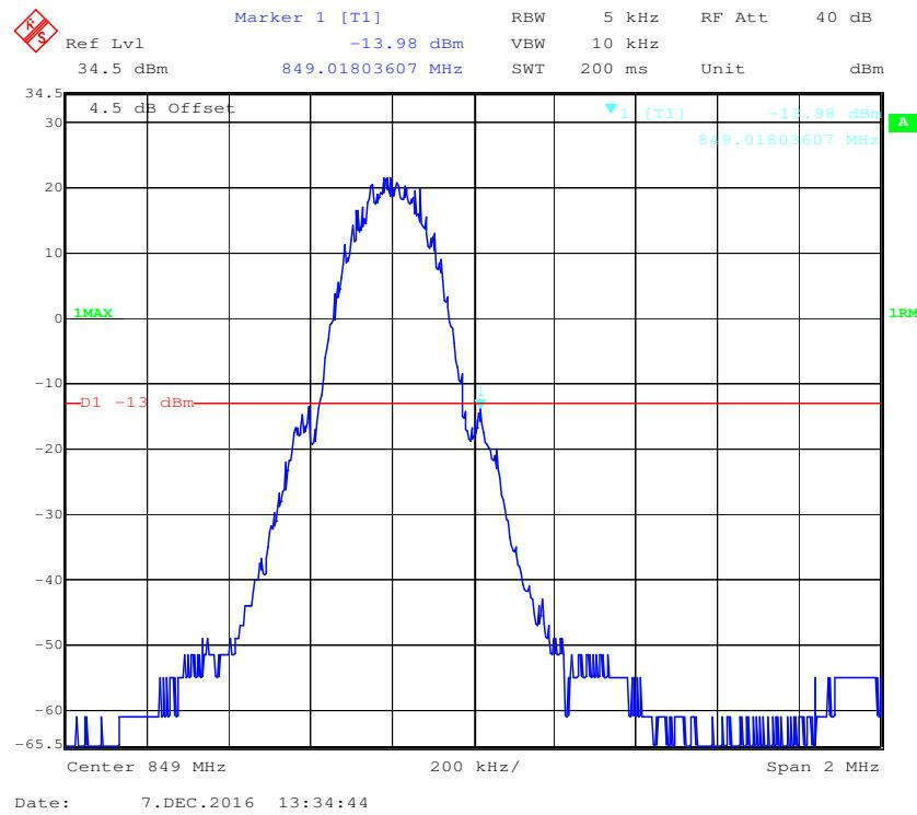
**Cellular Band, Left Band Edge for EDGE Mode**
