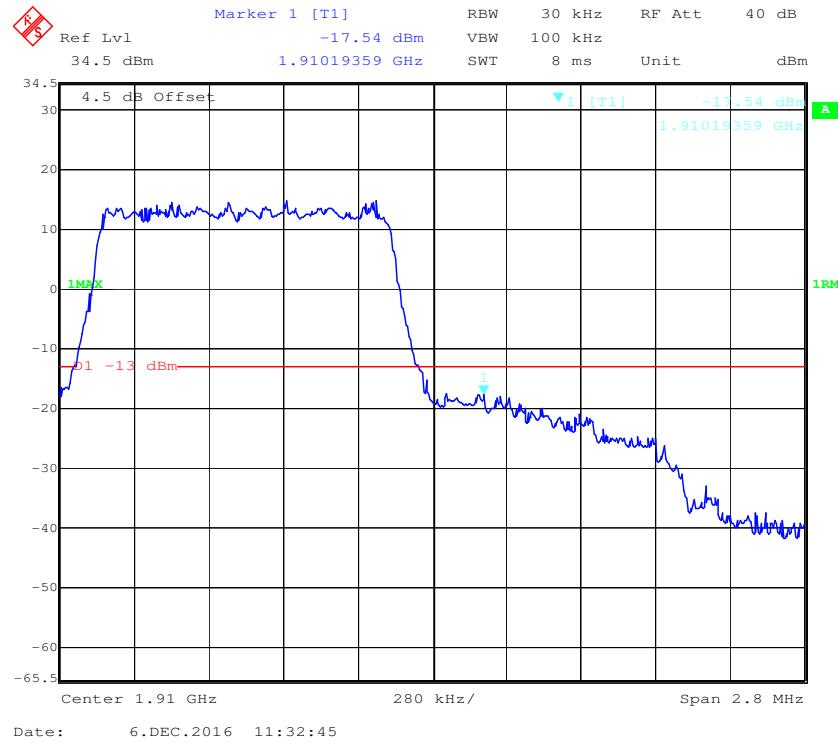
**16-QAM (1.4 MHz, FULL RB) - Left Band Edge**
