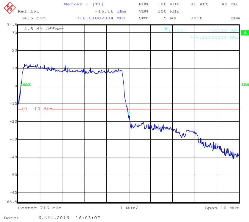
**QPSK (10.0 MHz, FULL RB) - Left Band Edge**
