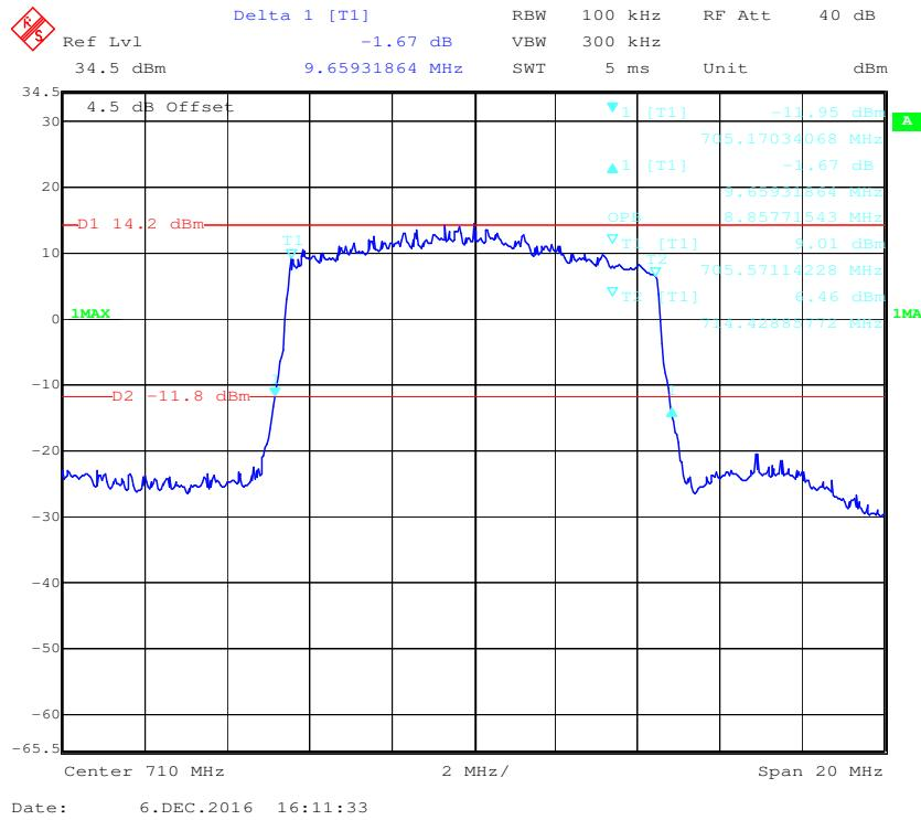
**16-QAM (10.0 MHz) - 99% Occupied Bandwidth &26 dB Bandwidth, Middle channel**
