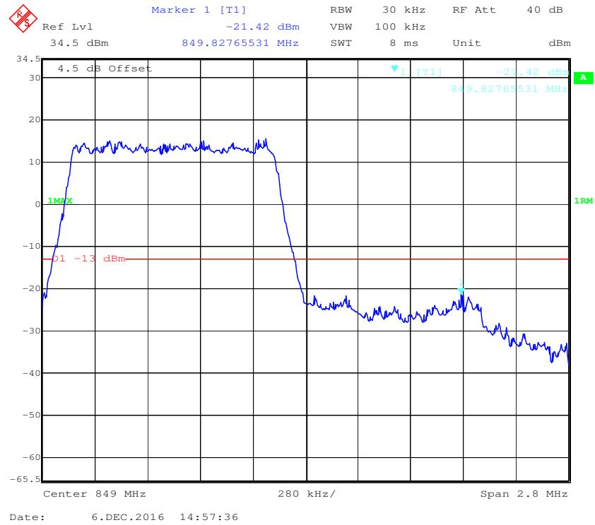
**16-QAM (1.4 MHz, FULL RB) - Left Band Edge**
