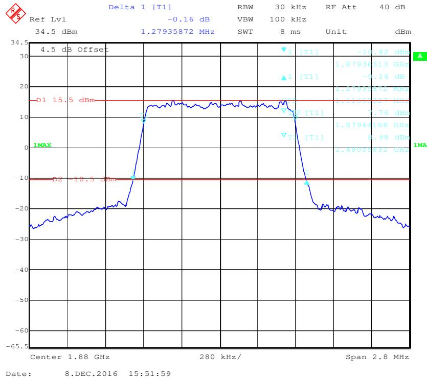
**16-QAM (1.4 MHz) - 99% Occupied Bandwidth &26 dB Bandwidth, Middle channel**
