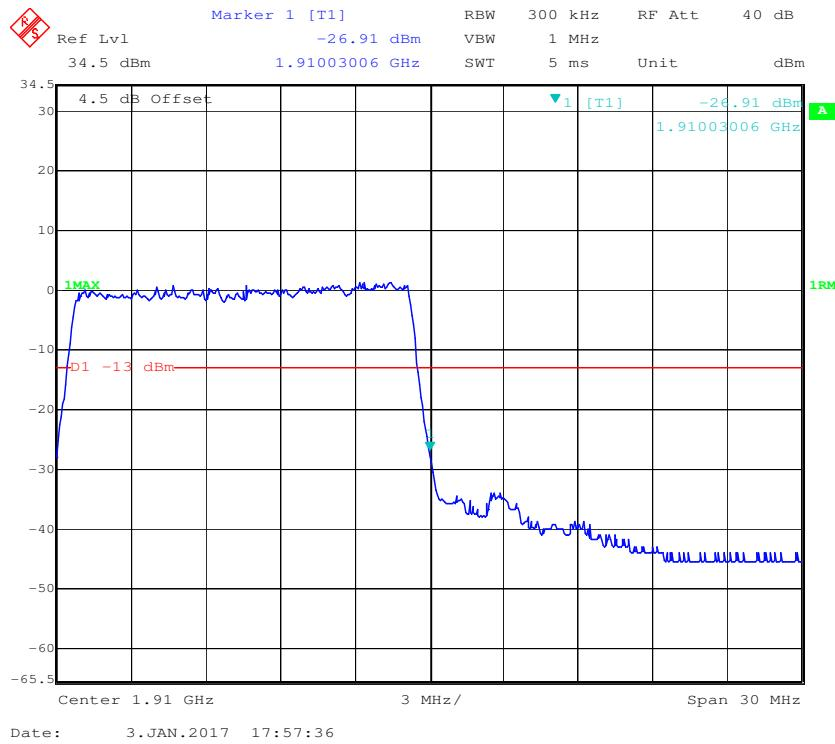
**16-QAM (15.0 MHz, FULL RB) - Left Band Edge**
