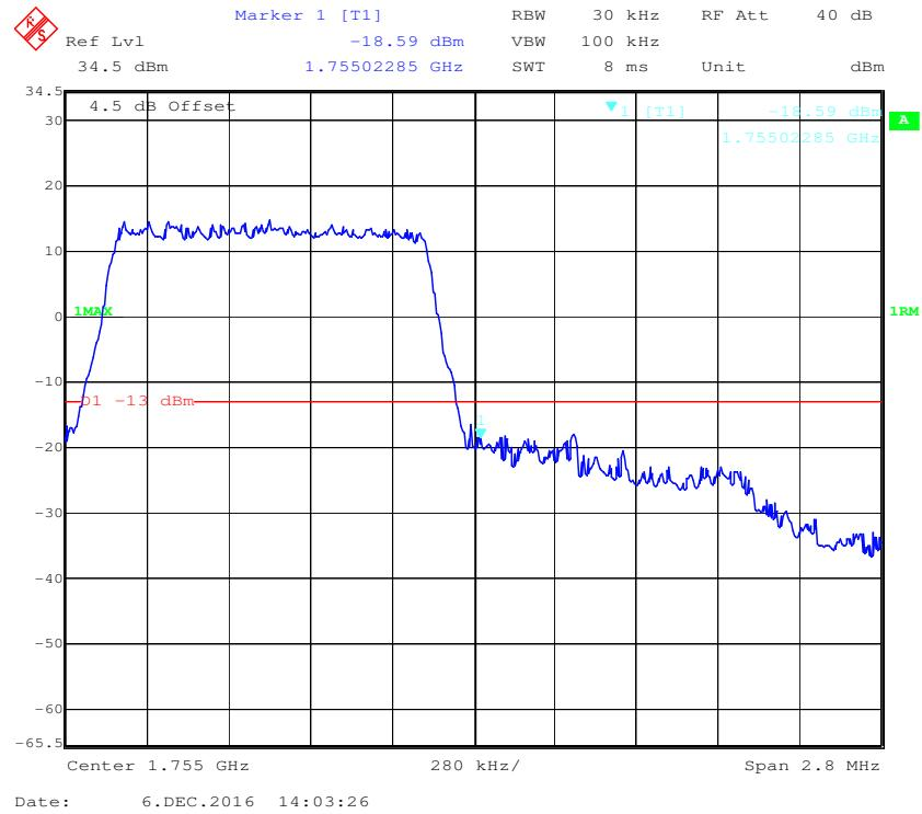
**16-QAM (1.4 MHz, FULL RB) - Left Band Edge**
