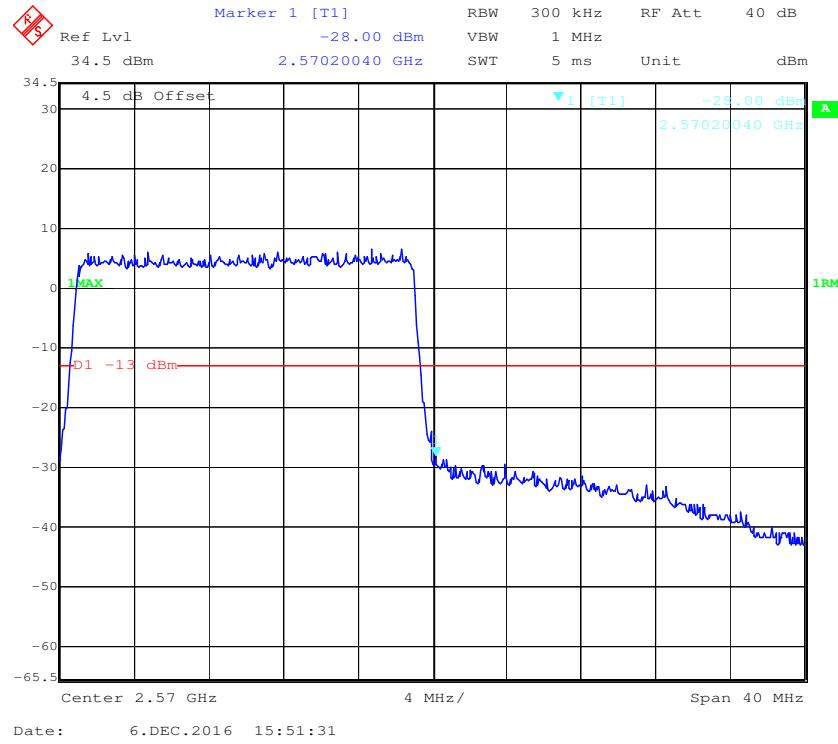
**LTE Band 17:****QPSK (5.0 MHz, FULL RB) - Left Band Edge**
