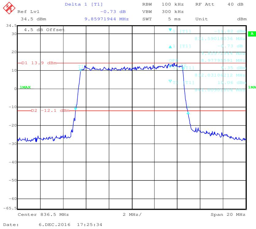
**16-QAM (10.0 MHz) - 99% Occupied Bandwidth & 26 dB Bandwidth, Middle channel**
