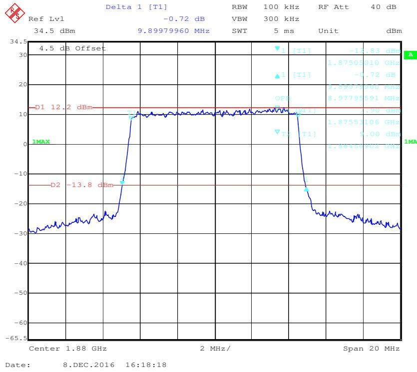
**16-QAM (10.0 MHz) - 99% Occupied Bandwidth &26 dB Bandwidth, Middle channel**
