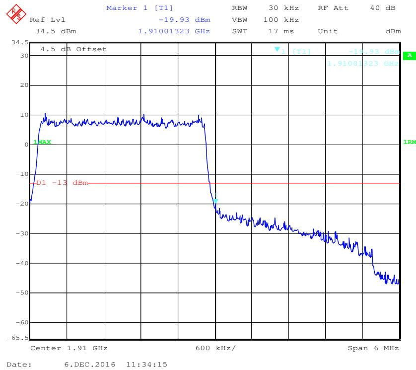
**16-QAM (3.0 MHz, FULL RB) - Left Band Edge**
