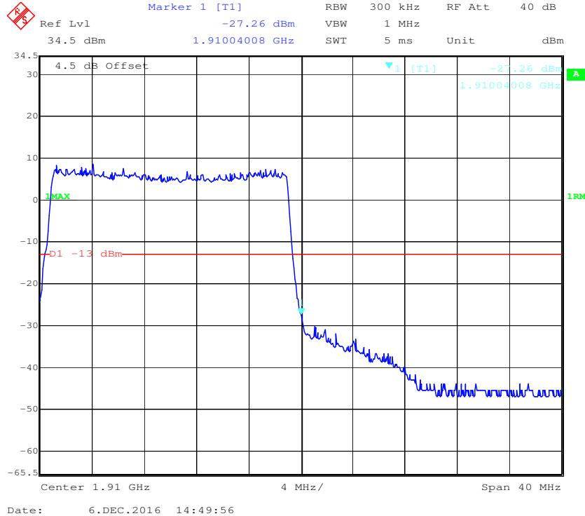
**LTE Band 4:****QPSK (1.4 MHz, FULL RB) - Left Band Edge**
