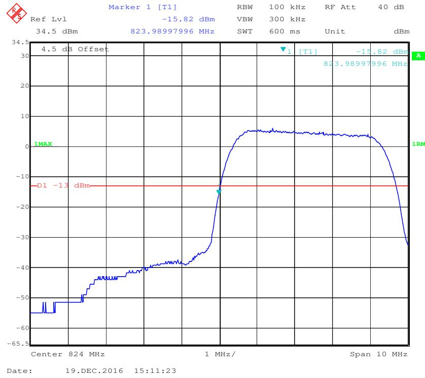
**Cellular Band, Right Band Edge for HSUPA (BPSK) Mode**
