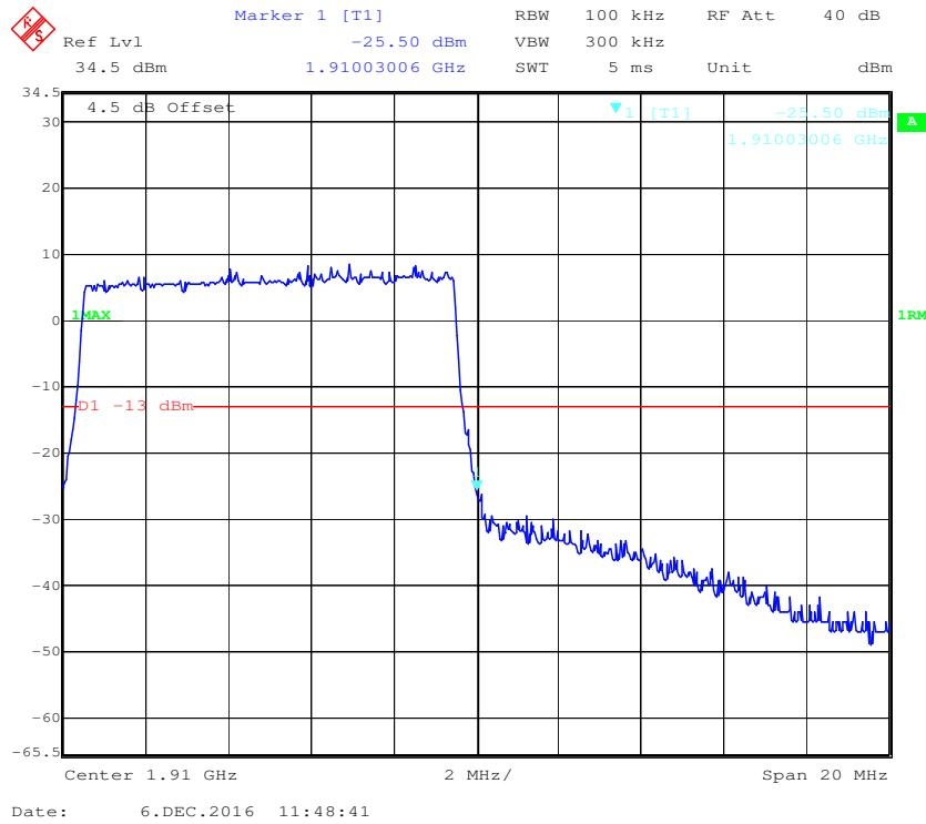
**QPSK (15.0 MHz, FULL RB) - Left Band Edge**
