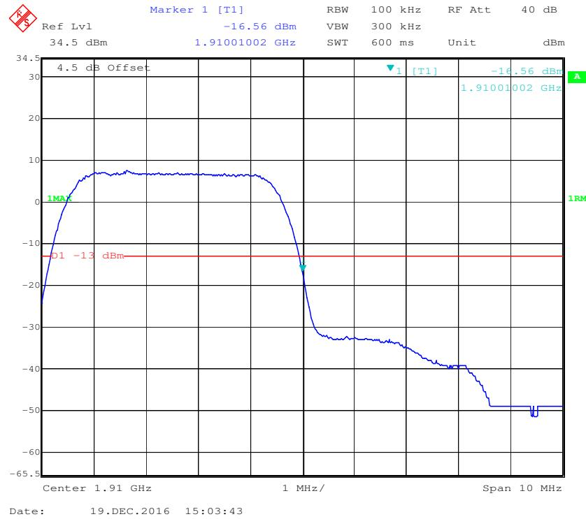
**AWS Band, Left Band Edge for RMC (BPSK) Mode**
