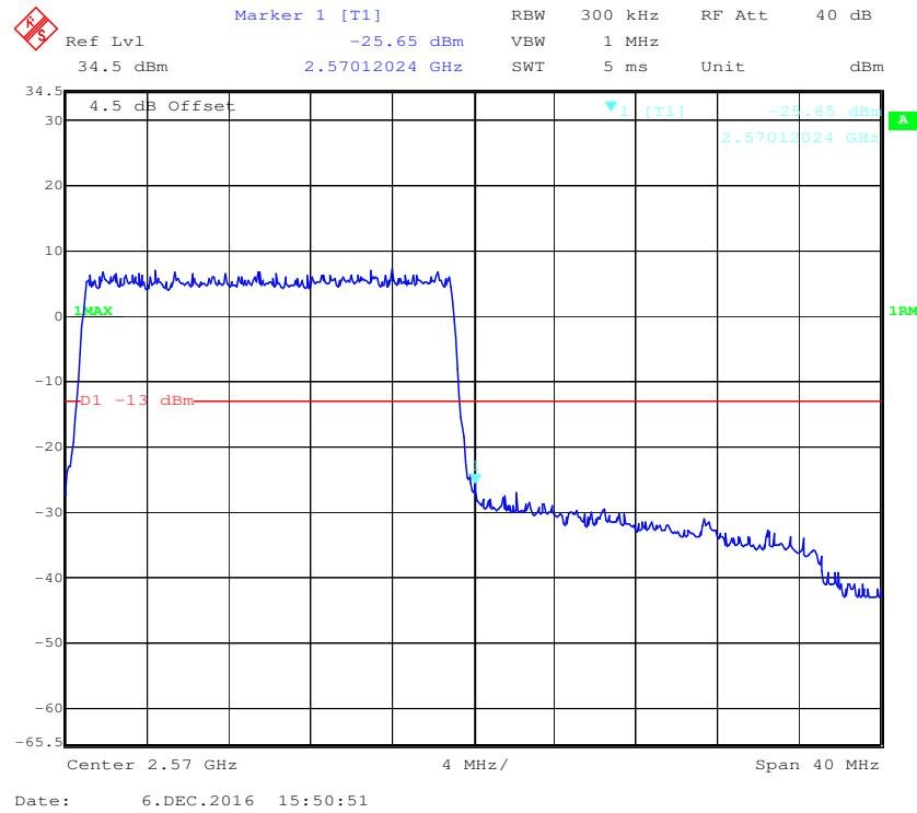
**16-QAM (20 MHz, FULL RB) - Left Band Edge**
