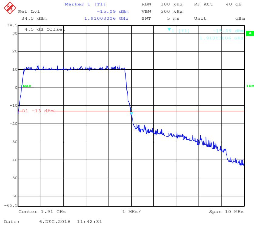
**16-QAM (5.0 MHz, FULL RB) - Left Band Edge**
