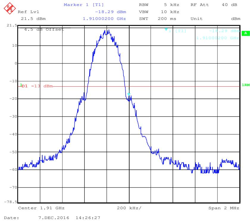
**PCS Band, Left Band Edge for EDGE Mode**
