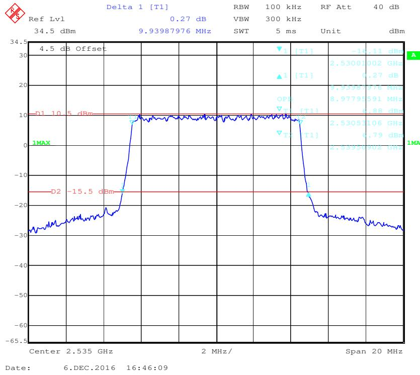
**16-QAM (10MHz) - 99% Occupied Bandwidth &26 dB Bandwidth, Middle channel**
