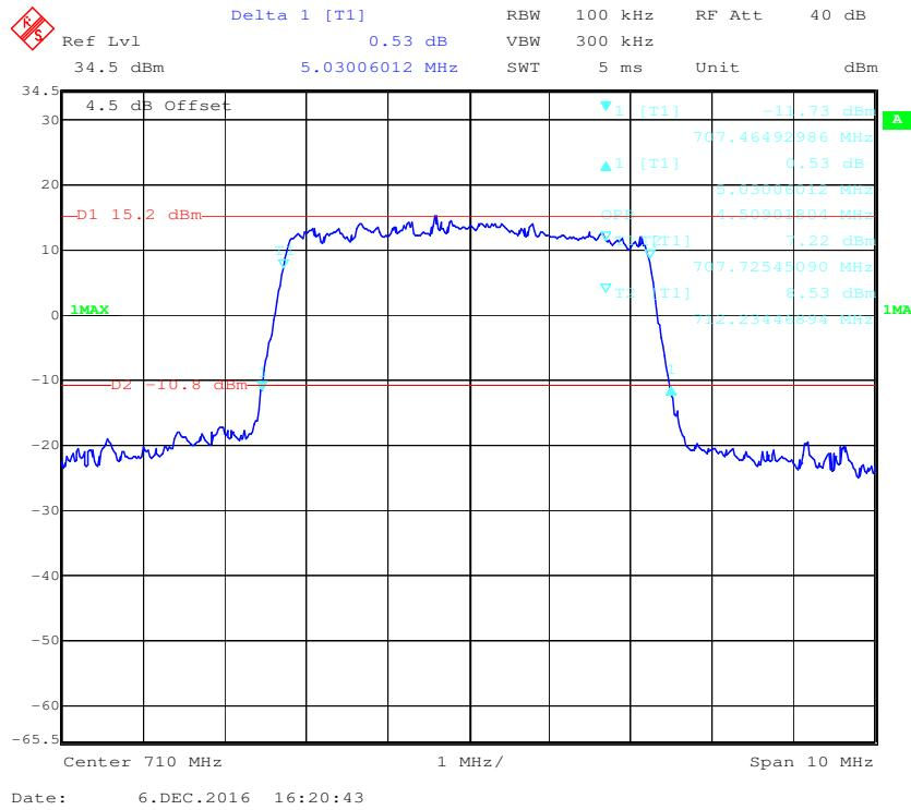
**16-QAM (5.0 MHz) - 99% Occupied Bandwidth &26 dB Bandwidth, Middle channel**
