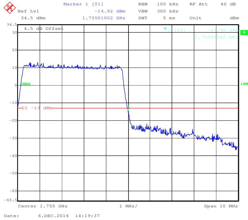
**QPSK (10.0 MHz, FULL RB) - Left Band Edge**
