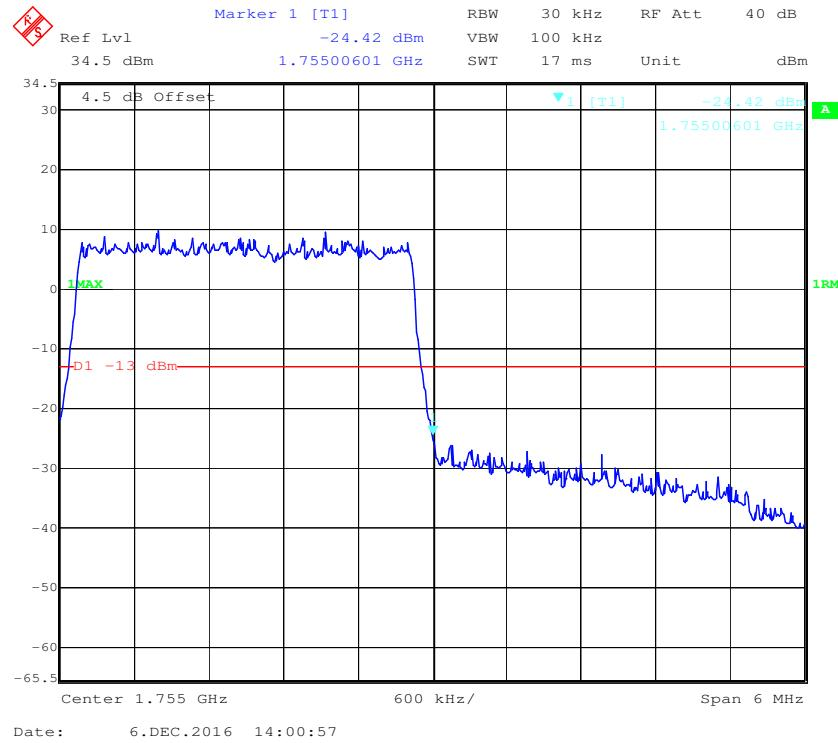
**QPSK (5.0 MHz, FULL RB) - Left Band Edge**
