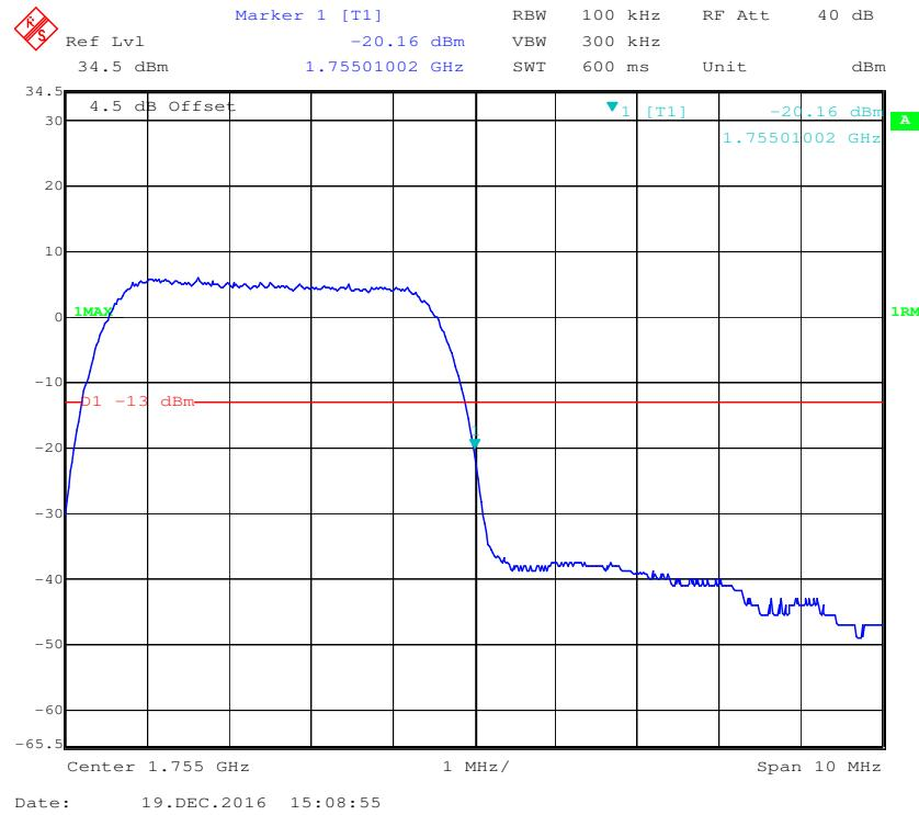
**AWS Band, Left Band Edge for HSUPA (BPSK) Mode**
