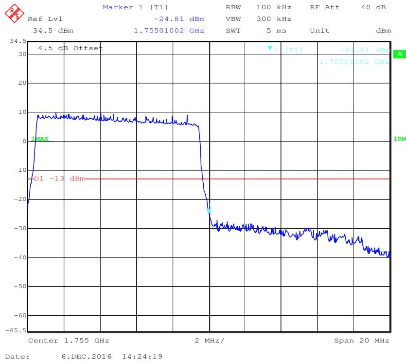
**QPSK (15.0 MHz, FULL RB) - Left Band Edge**
