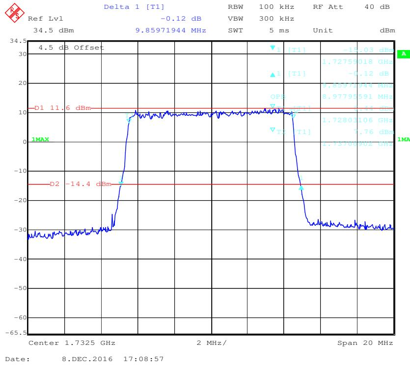
**16-QAM (10.0 MHz) - 99% Occupied Bandwidth &26 dB Bandwidth, Middle channel**
