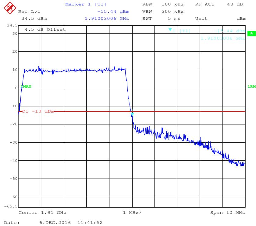
**QPSK (10.0 MHz, FULL RB) - Left Band Edge**
