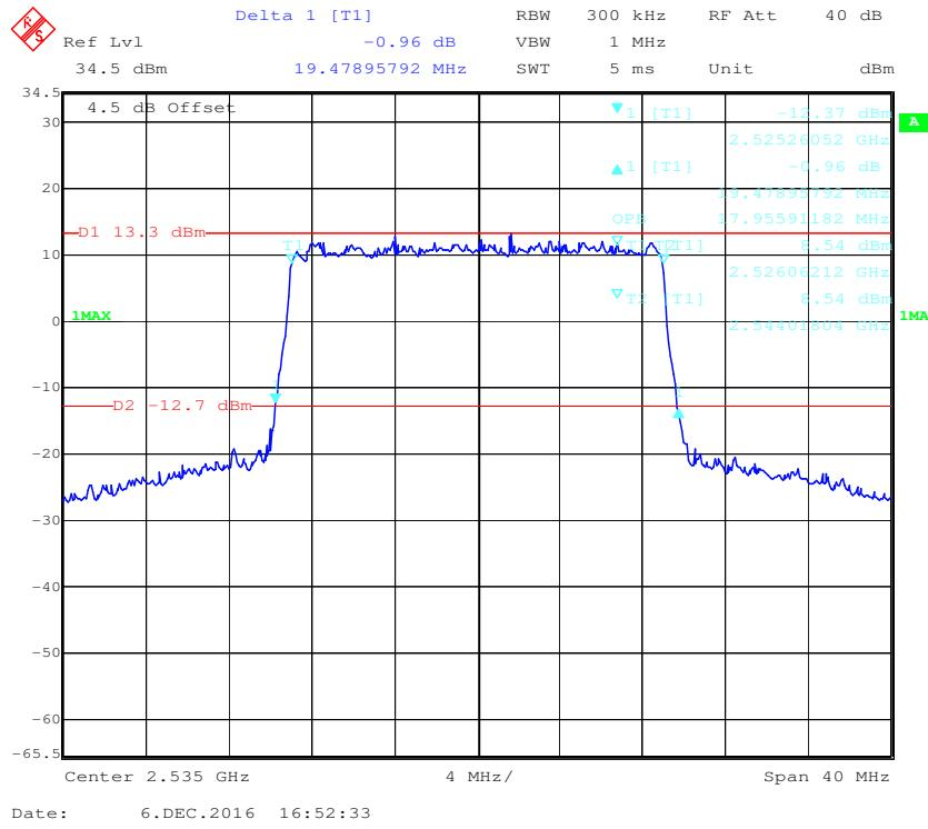
**16-QAM (20 MHz) - 99% Occupied Bandwidth &26 dB Bandwidth, Middle channel**
