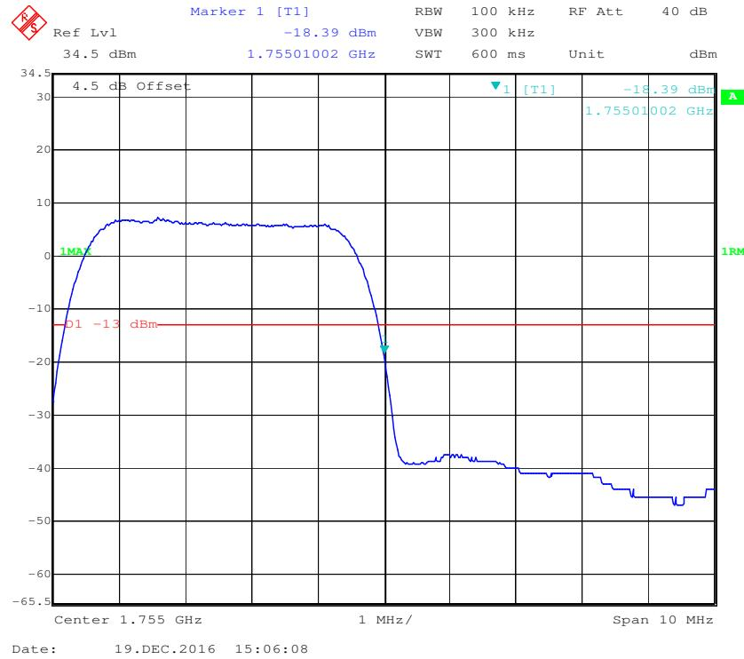
**AWS Band, Left Band Edge for HSDPA (16QAM) Mode**
