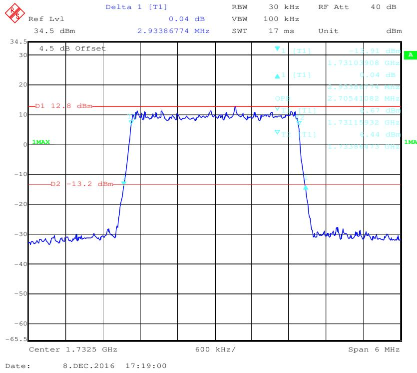
**16-QAM (3.0 MHz) - 99% Occupied Bandwidth &26 dB Bandwidth, Middle channel**
