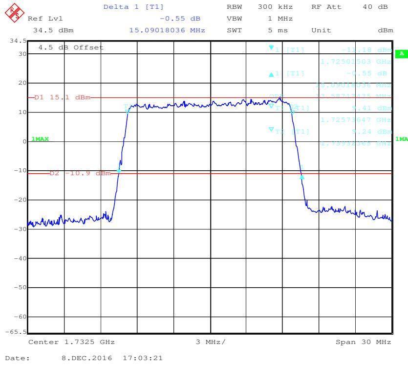
**16-QAM (15.0 MHz) - 99% Occupied Bandwidth &26 dB Bandwidth, Middle channel**
