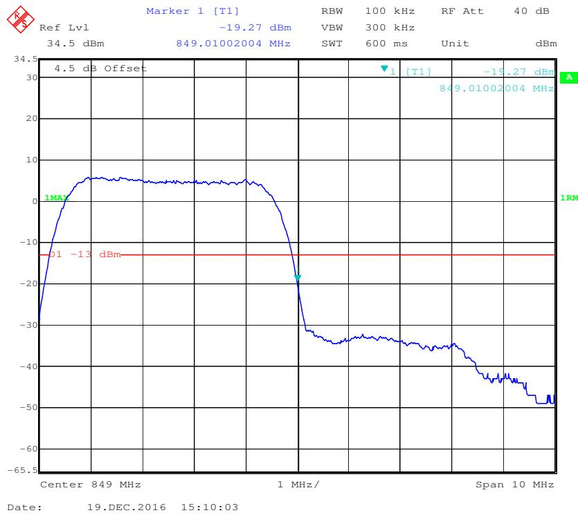
**Cellular Band, Left Band Edge for HSUPA (BPSK) Mode**
