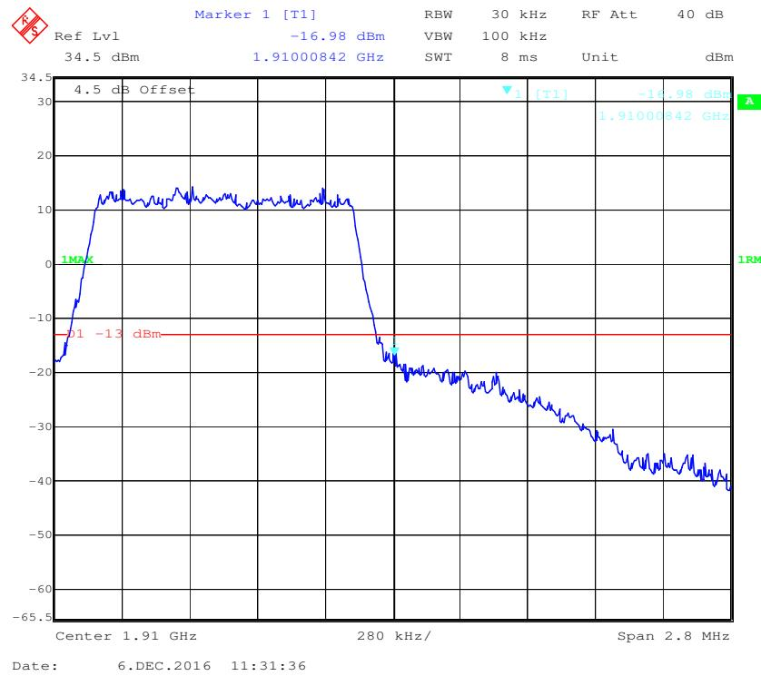
**QPSK (3.0 MHz, FULL RB) - Left Band Edge**
