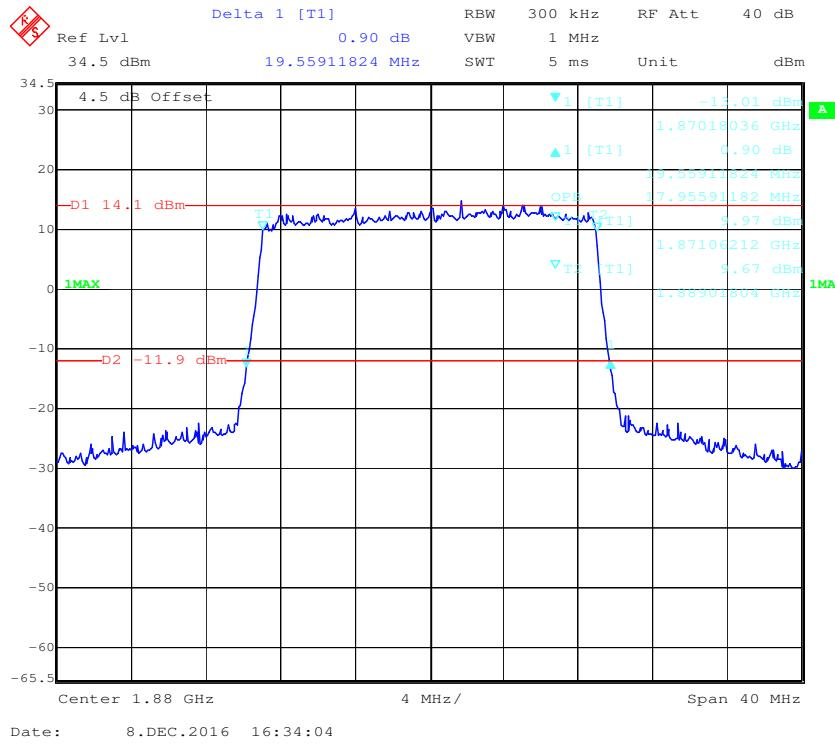
**16-QAM (20.0 MHz) - 99% Occupied Bandwidth & 26 dB Bandwidth, Middle channel**
