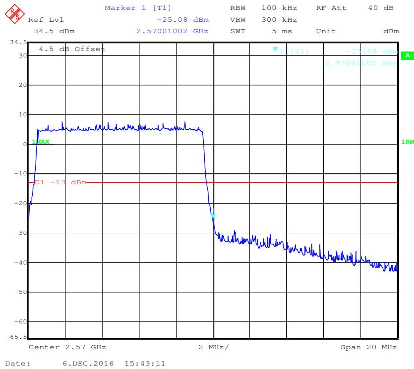
**QPSK (15 MHz, FULL RB) - Left Band Edge**
