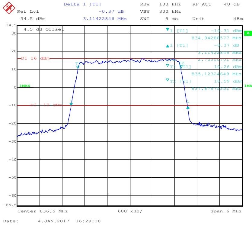
**16-QAM (3.0 MHz) - 99% Occupied Bandwidth &26 dB Bandwidth, Middle channel**
