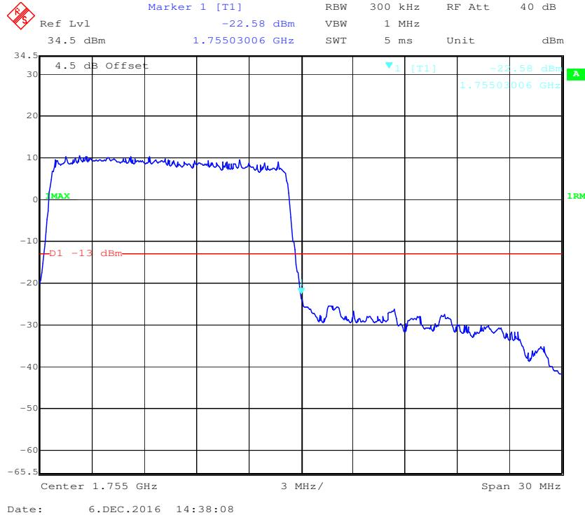
**16-QAM (15.0 MHz, FULL RB) - Left Band Edge**
