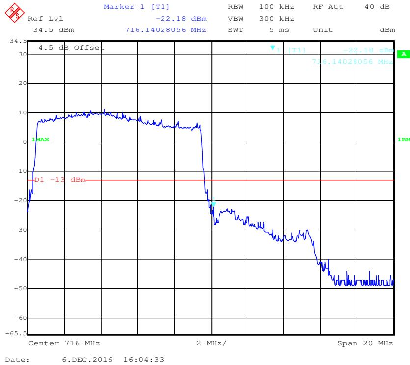
**16-QAM (10.0 MHz, FULL RB) - Left Band Edge**
