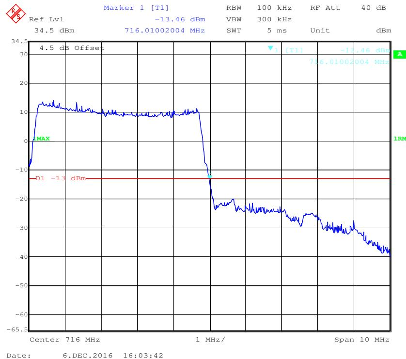
**16-QAM (5.0 MHz, FULL RB) - Left Band Edge**
