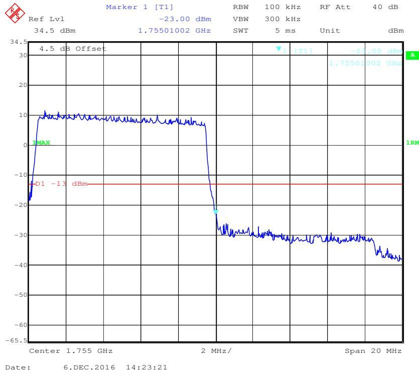
**16-QAM (10.0 MHz, FULL RB) - Left Band Edge**
