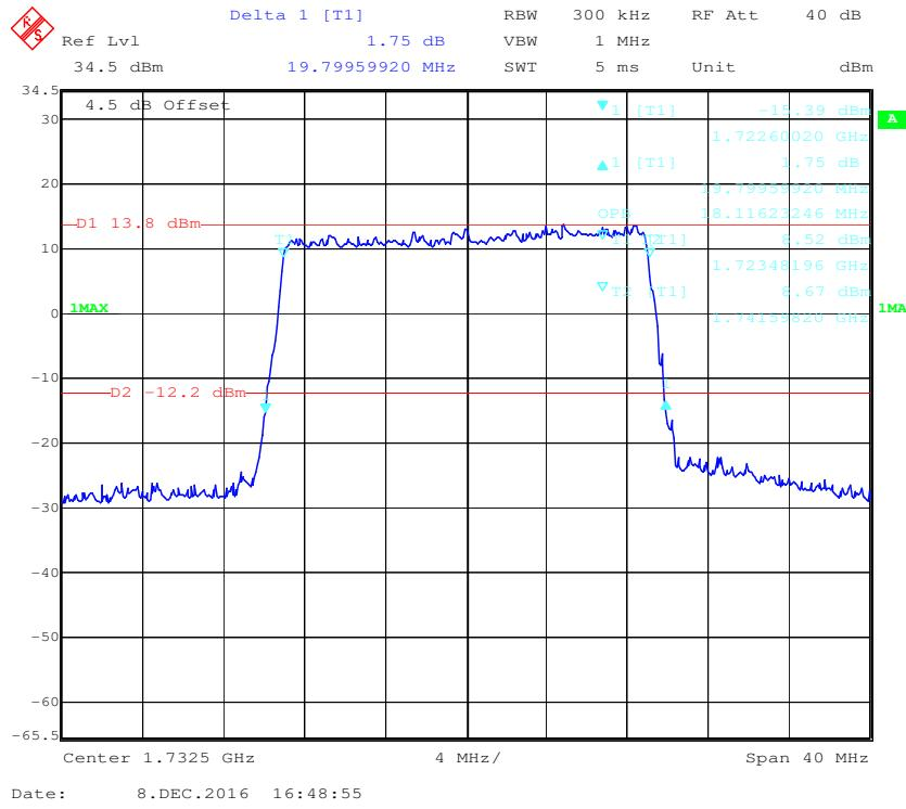
**16-QAM (20.0 MHz) - 99% Occupied Bandwidth &26 dB Bandwidth, Middle channel**
