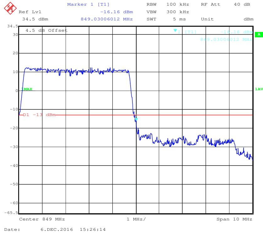
**16-QAM (5.0 MHz, FULL RB) - Left Band Edge**
