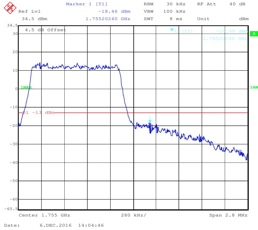
**QPSK (3.0 MHz, FULL RB) - Left Band Edge**
