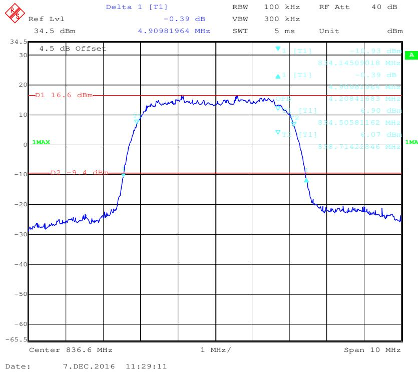
**PCS Band (Part 24E)****26 dB Emissions &99% Occupied Bandwidth for GSM (GMSK) Mode**
