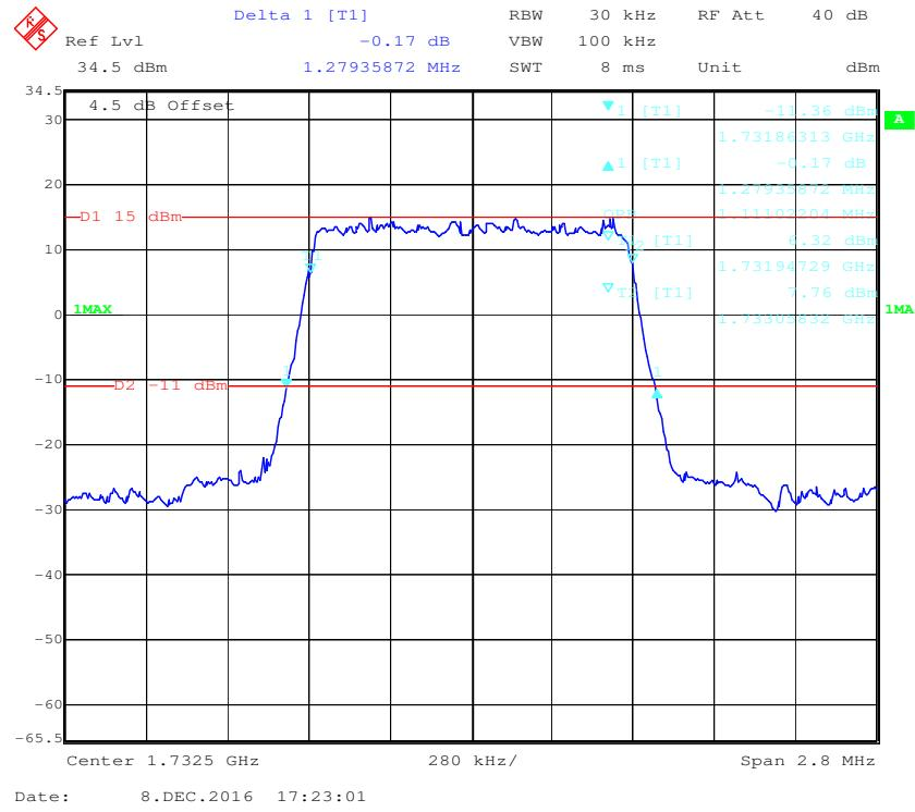
**16-QAM (1.4 MHz) - 99% Occupied Bandwidth &26 dB Bandwidth, Middle channel**
