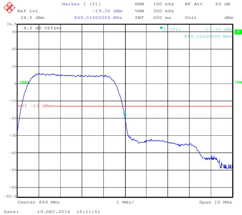
**PCS Band, Left Band Edge for GSM (GMSK) Mode**
