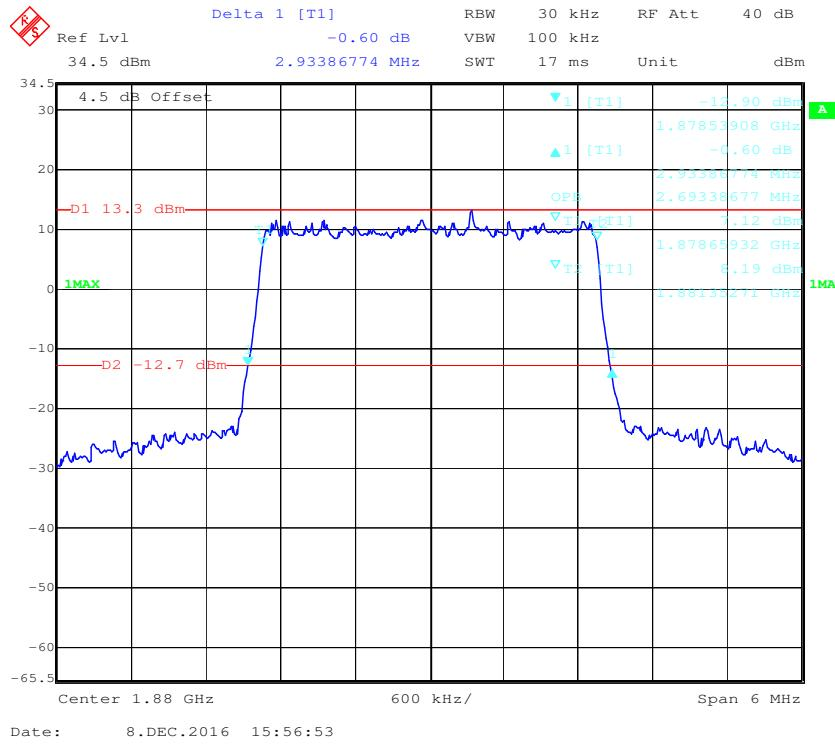
**16-QAM (3.0 MHz) - 99% Occupied Bandwidth &26 dB Bandwidth, Middle channel**
