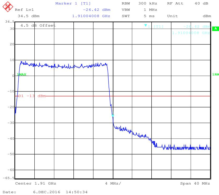
**16-QAM (20.0 MHz, FULL RB) - Left Band Edge**
