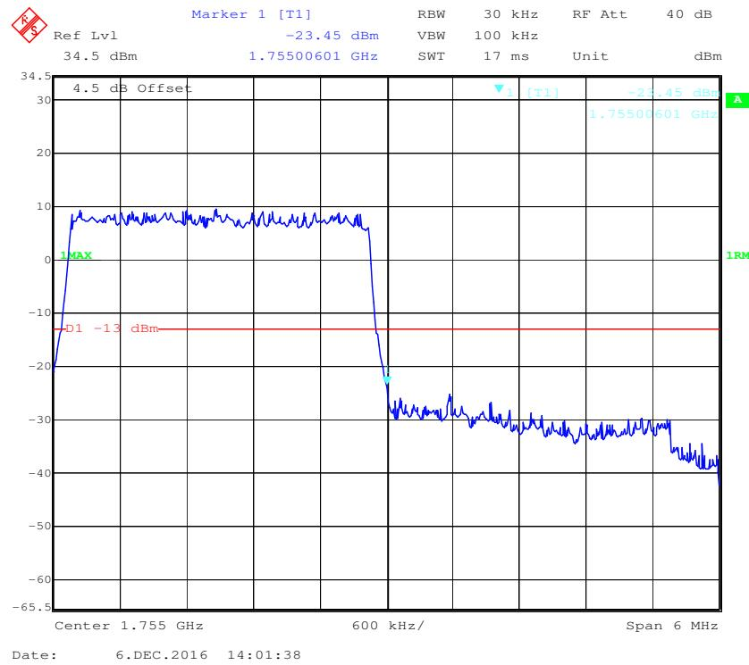
**16-QAM (3.0 MHz, FULL RB) - Left Band Edge**
