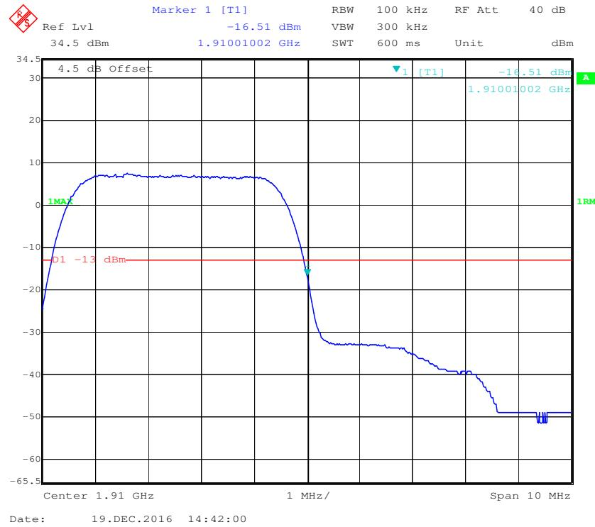
**PCS Band, Left Band Edge for HSDPA (16QAM) Mode**
