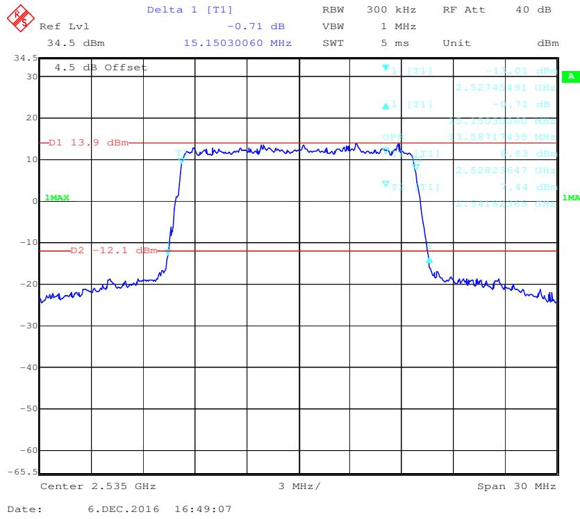
**16-QAM (15 MHz) - 99% Occupied Bandwidth &26 dB Bandwidth, Middle channel**
