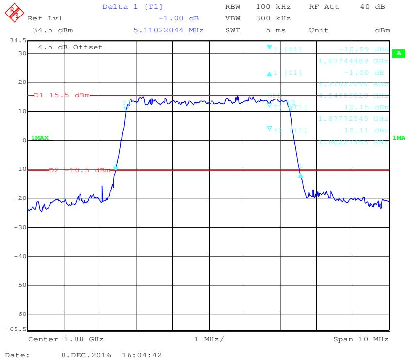
**16-QAM (5.0 MHz) - 99% Occupied Bandwidth &26 dB Bandwidth, Middle channel**
