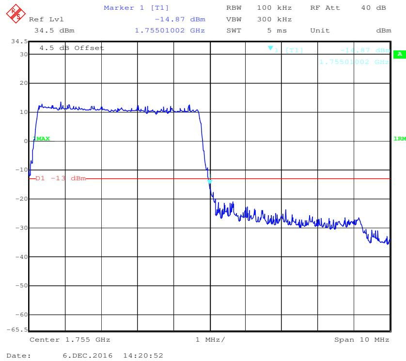
**16-QAM (5.0 MHz, FULL RB) - Left Band Edge**
