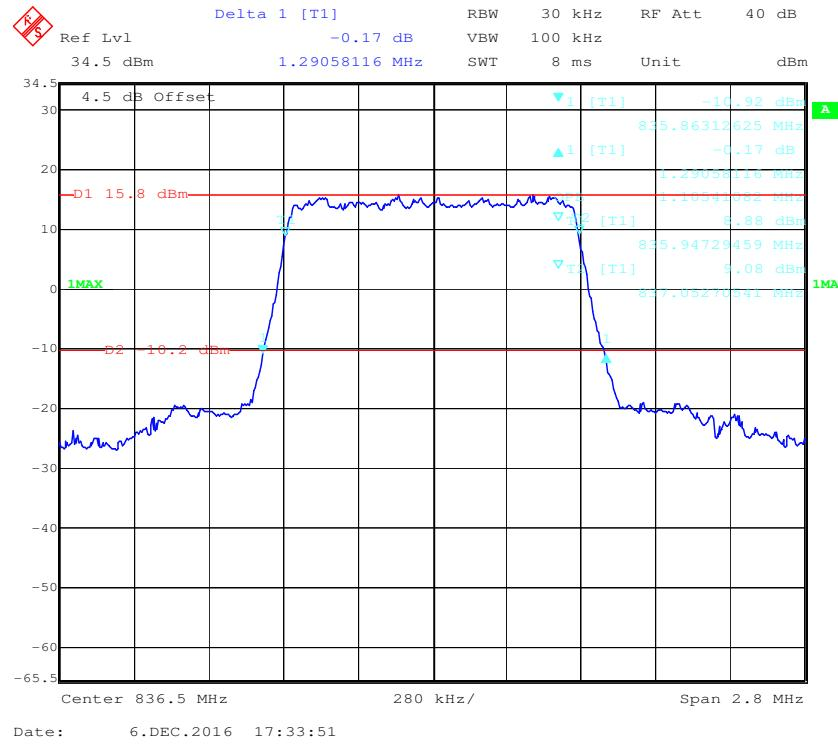
**16-QAM (1.4 MHz) - 99% Occupied Bandwidth &26 dB Bandwidth, Middle channel**
