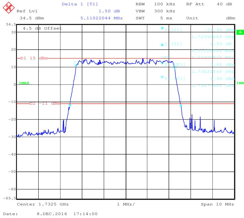
**16-QAM (5.0 MHz) - 99% Occupied Bandwidth &26 dB Bandwidth, Middle channel**
