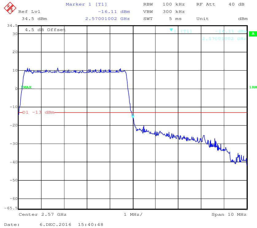
**16-QAM (5.0 MHz, FULL RB) - Left Band Edge**
