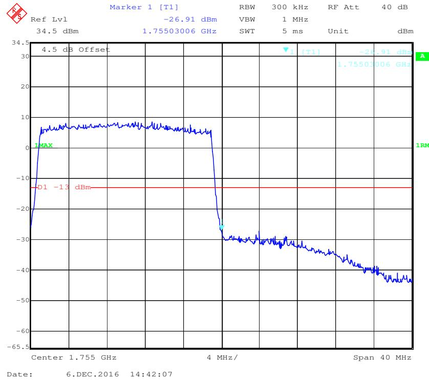
**LTE Band 5:****QPSK (1.4 MHz, FULL RB) - Left Band Edge**
