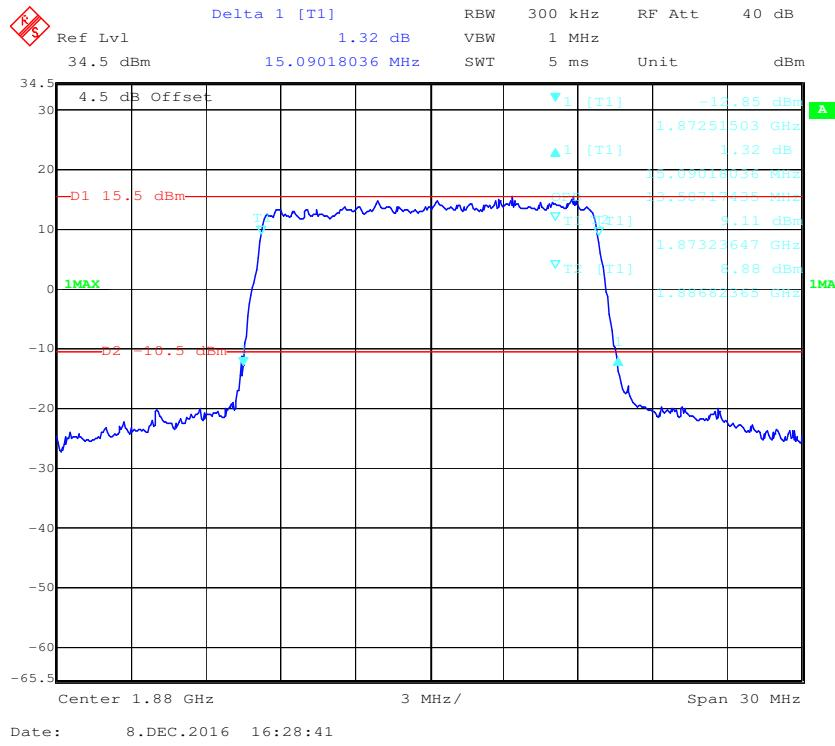
**16-QAM (15.0 MHz) - 99% Occupied Bandwidth &26 dB Bandwidth, Middle channel**
