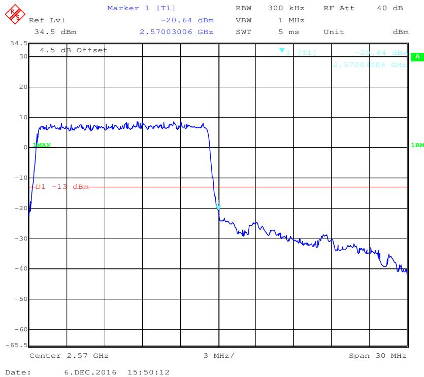
**16-QAM (15 MHz, FULL RB) - Left Band Edge**
