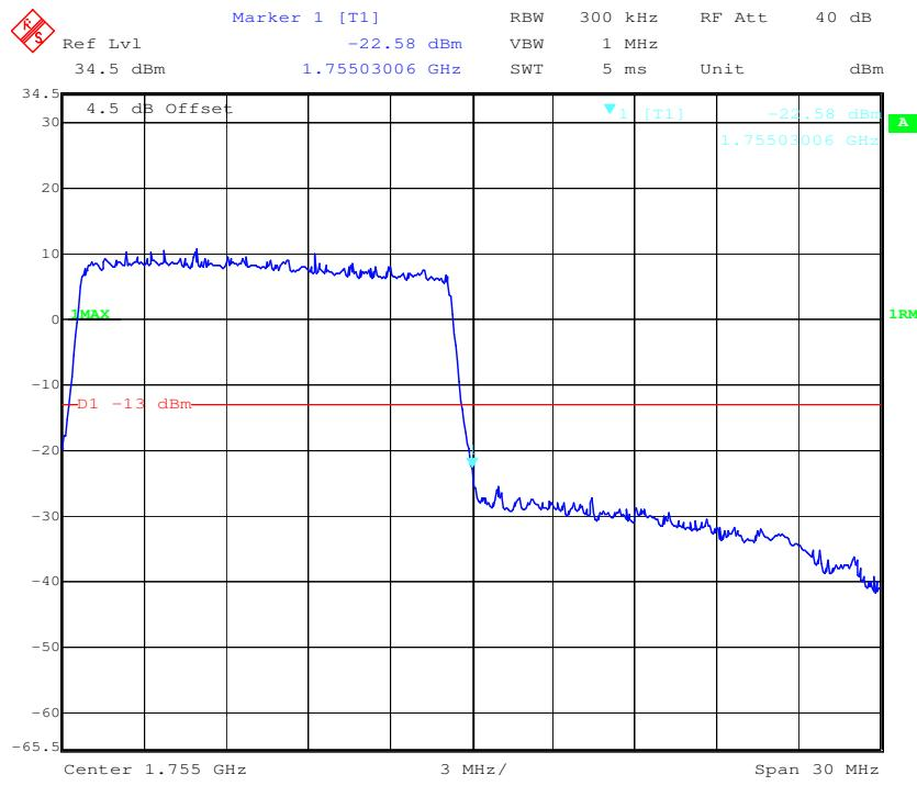
**QPSK (20.0 MHz, FULL RB) - Left Band Edge**
