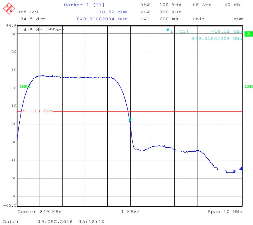
**Cellular Band, Left Band Edge for HSDPA (16QAM) Mode**
