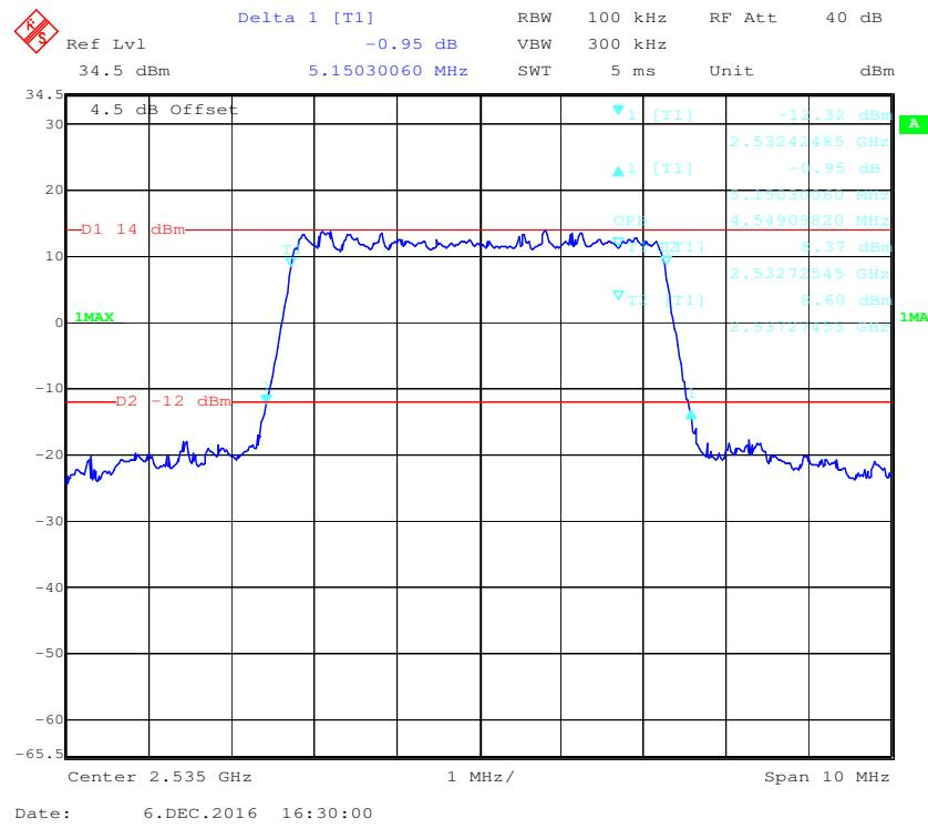
**16-QAM (5 MHz) - 99% Occupied Bandwidth &26 dB Bandwidth, Middle channel**
