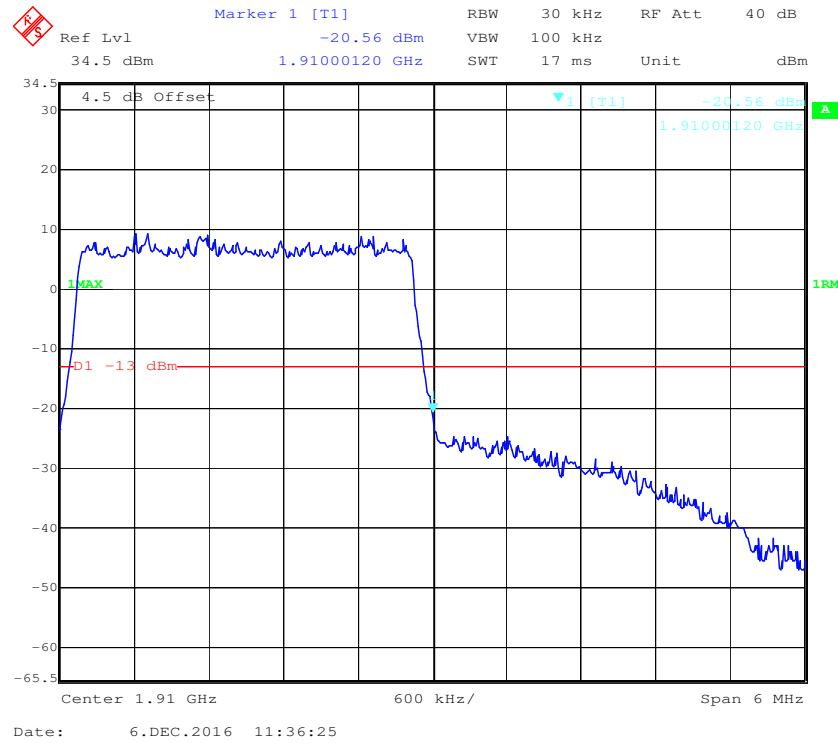
**QPSK (5.0 MHz, FULL RB) - Left Band Edge**
