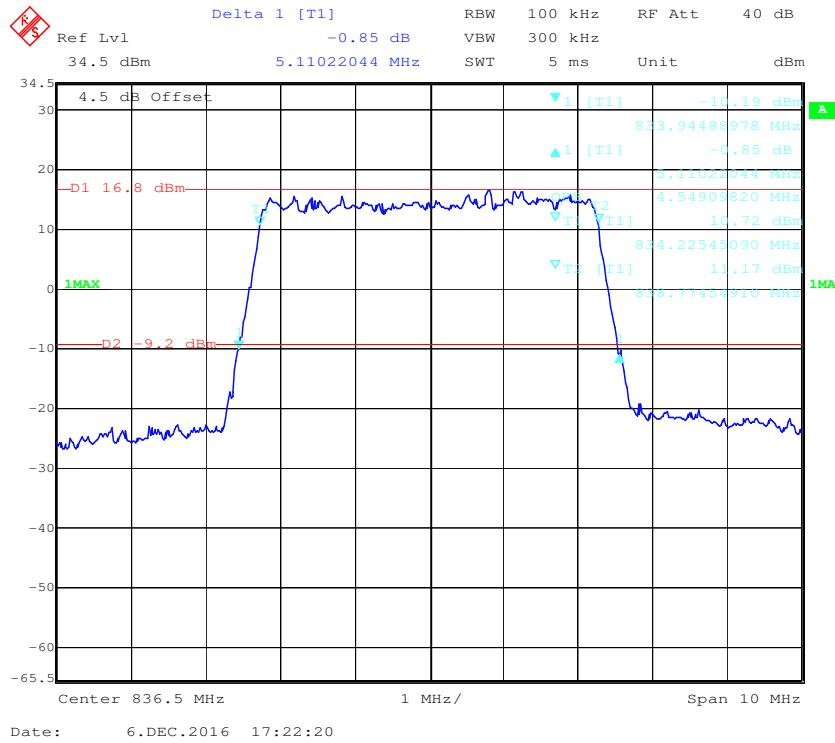
**16-QAM (5.0 MHz) - 99% Occupied Bandwidth &26 dB Bandwidth, Middle channel**
