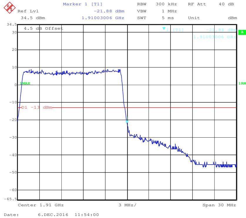
**QPSK (20.0 MHz, FULL RB) - Left Band Edge**
