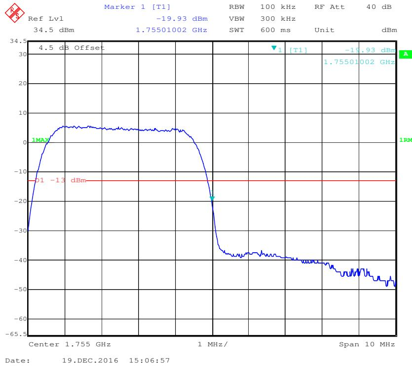
**LTE Band 2:****QPSK (1.4 MHz, FULL RB) - Left Band Edge**
