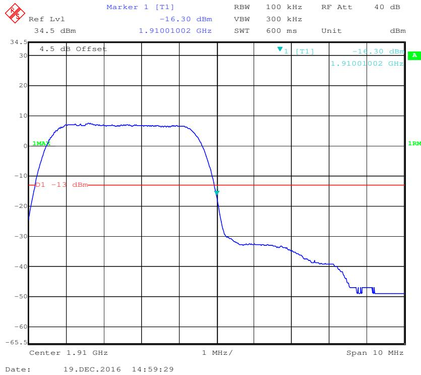
**PCS Band, Left Band Edge for HSUPA (BPSK) Mode**
