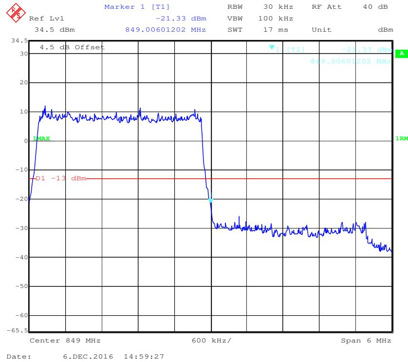
**16-QAM (3.0 MHz, FULL RB) - Left Band Edge**
