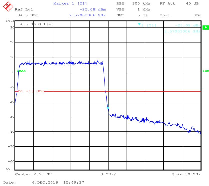
**QPSK (20 MHz, FULL RB) - Left Band Edge**
