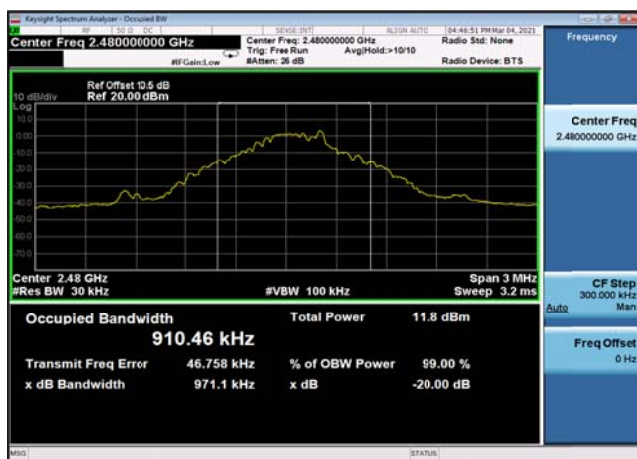
20dB Bandwidth: DQPSK,2441MHz,2DH5
