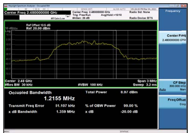
20dB Bandwidth: DQPSK,2480MHz,2DH5
