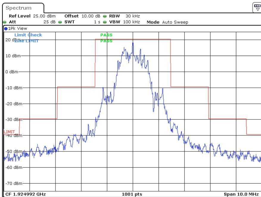
**High Channel (Unwanted Emission inside the Sub-band)**
