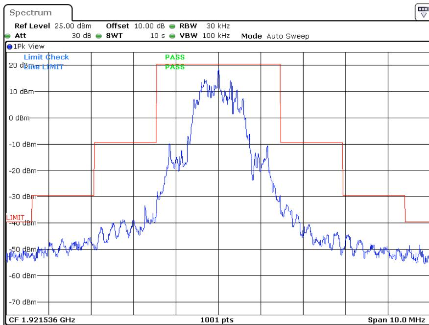
**Middle Channel (Unwanted Emission inside the Sub-band)**
