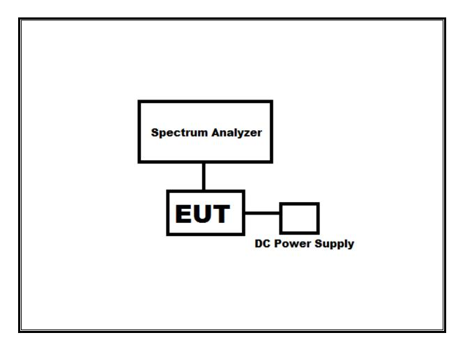
Note – The DC power supply is used only during testing. During normal operation the EUT is powered by a supplied CR2032, coin cell battery.
