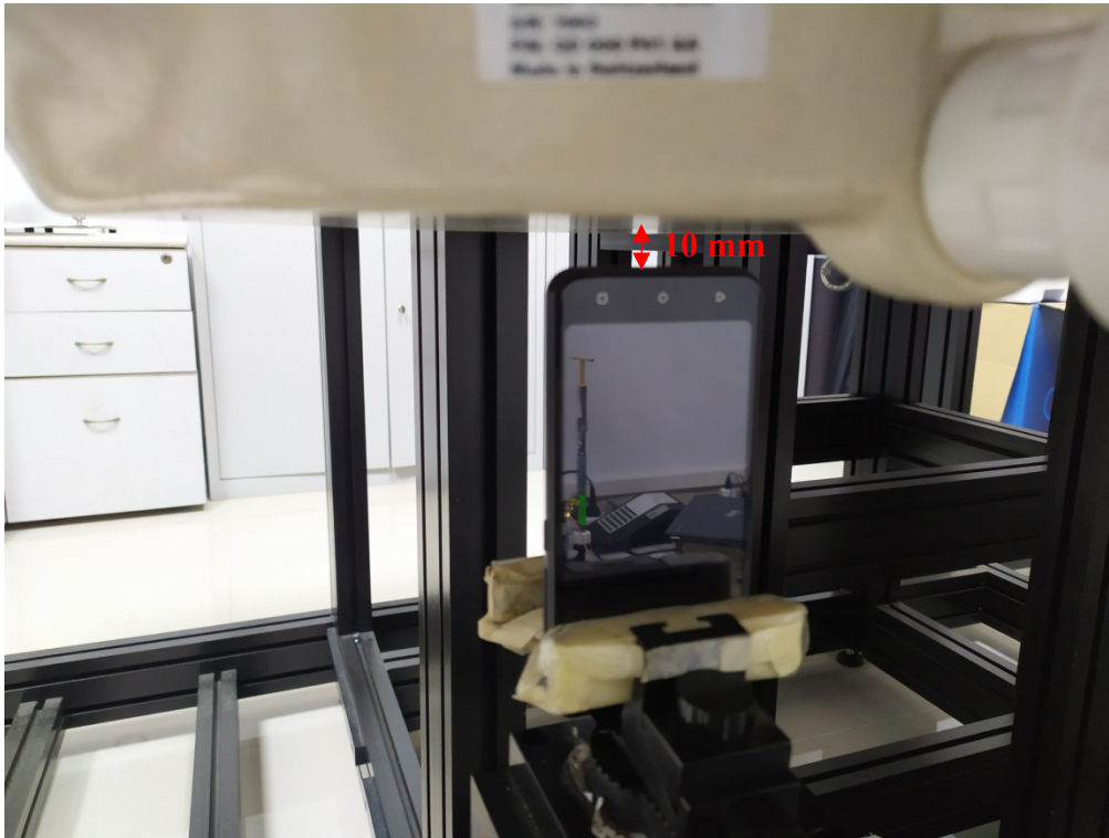
Body Bottom Setup Photo (10mm)
