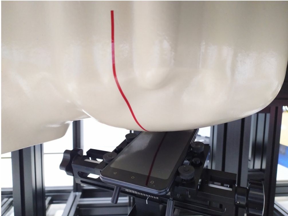
Head Right Cheek Setup Photo
