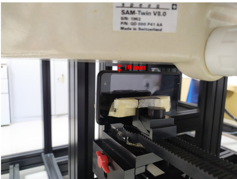
Body Left Setup Photo (10mm)
