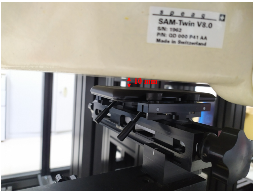
Body (Worn) Back Setup Photo (10mm)
