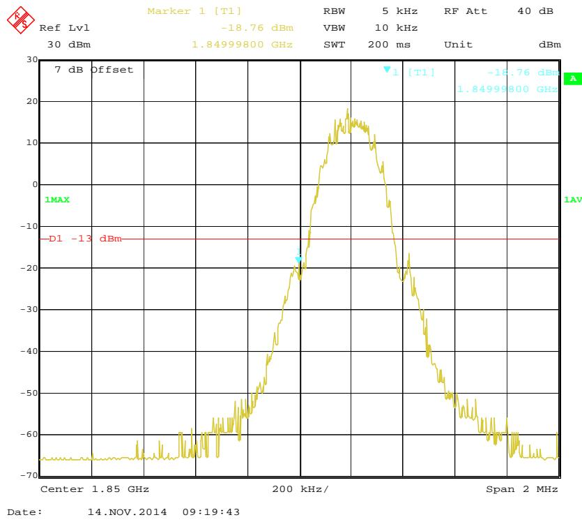
**PCS Band, Right Band Edge for GSM (GMSK) Mode**
