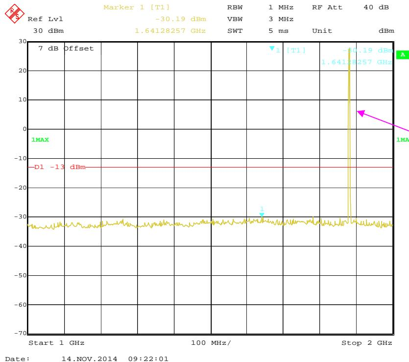
Fundamental test with notch filter
