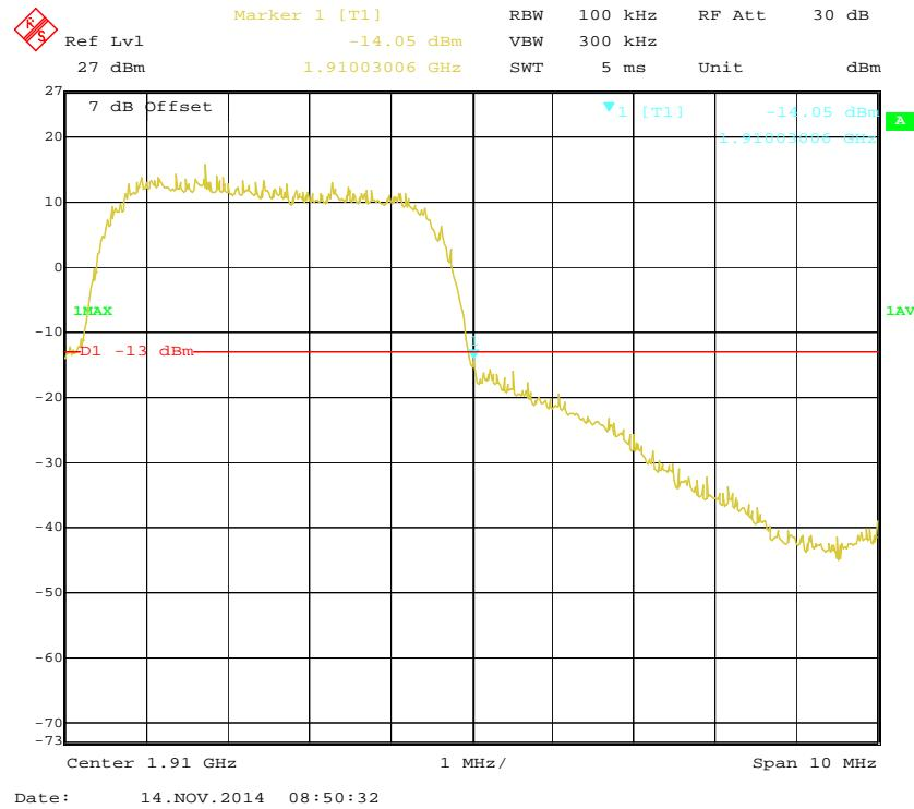
**PCS Band, Left Band Edge for HSDPA (16QAM) Mode**
