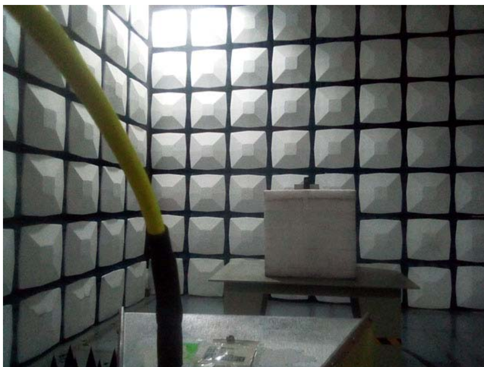
Radiated Emission Above 1GHz View
