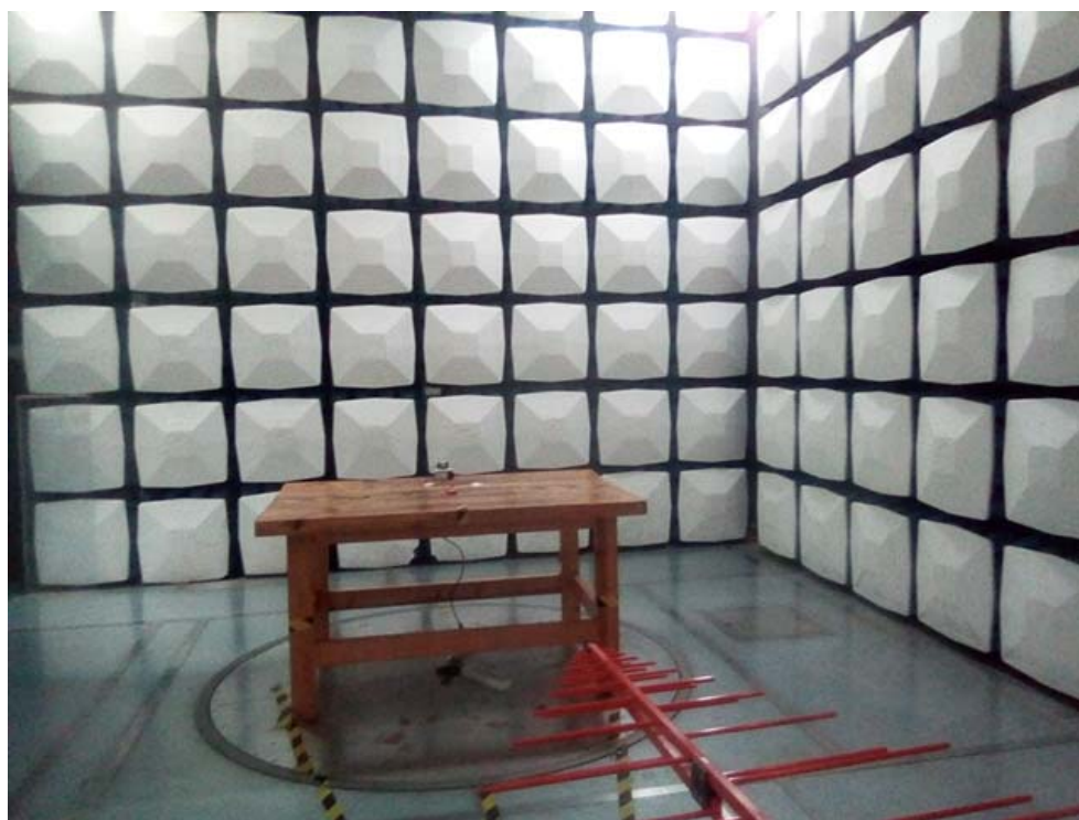
Radiated Emission Below 1GHz View
