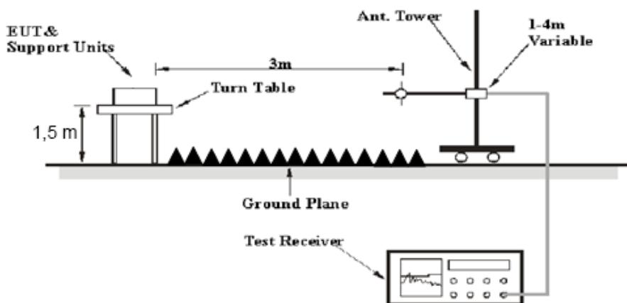
The radiated emission below 1GHz tests were performed in the 3 meters chamber A, above 1GHz tests were performed in the 3 meters chamber A, using the setup accordance with the ANSI C63.10-2013. The specification used was the FCC 15.209, and FCC 15.247 limits.
