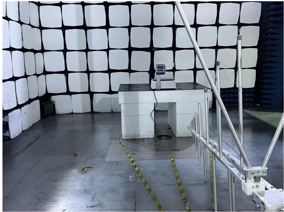
Radiation Emission Test Setup (30MHz to 1GHz)
