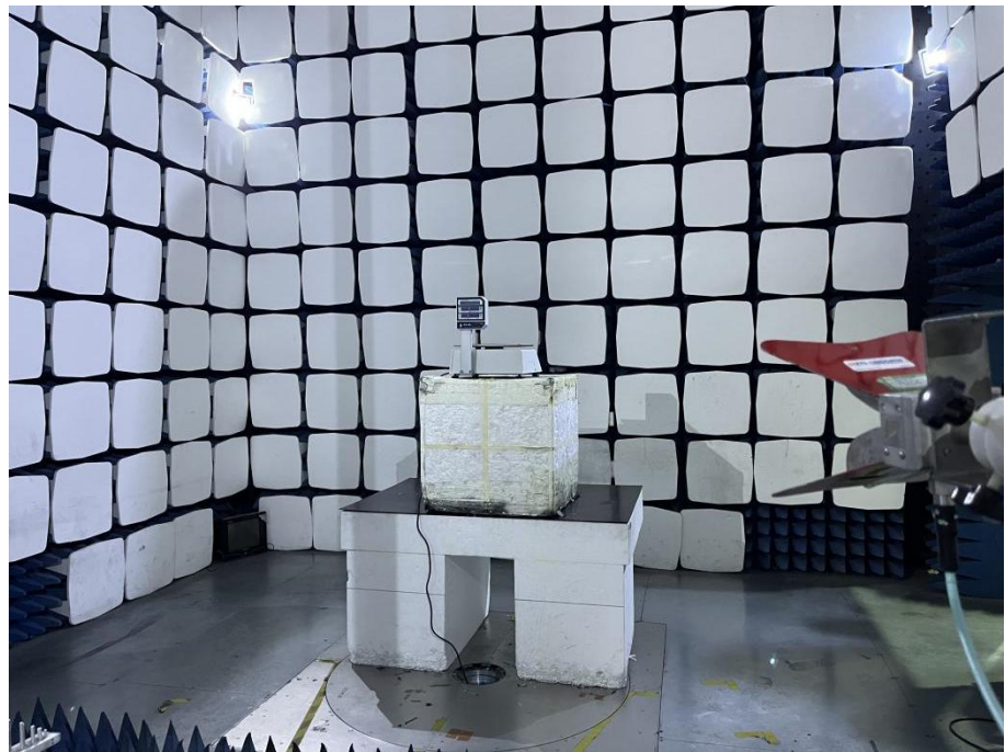
Radiation Emission Test Setup (1GHz to 18GHz)
