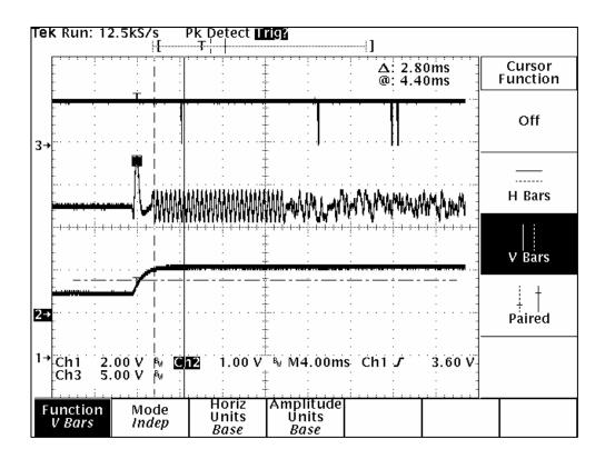
The recovered modulation should be centered at approximately 2.5 VDC and should have an amplitude of approximately 800 mV peal-to-peak as indicated in the plot above.
