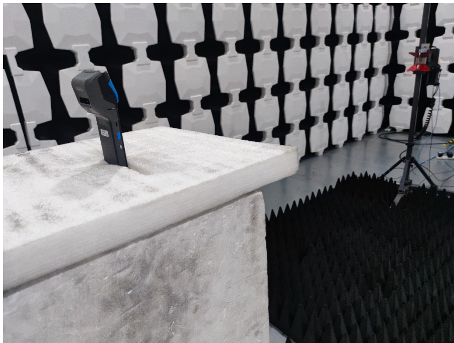
Description: Back view of Radiated Emission Test Setup (1GHz -18GHz)
