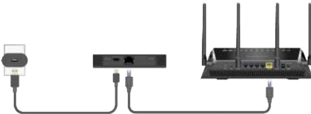
Figure 3. Ethernet offloading with AC charging and a USB storage device
