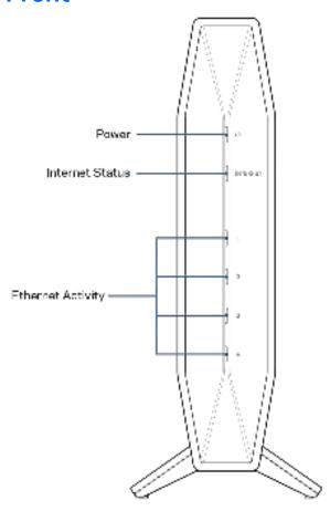
**Power light-**Blinks blue while router is starting up and during WPS pairing. Blinks yellow if WPS pairing fails
