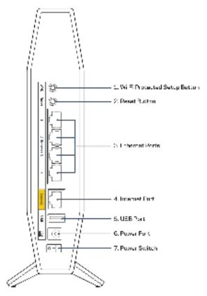
Wi-Fi Protected Setup™ (WPS) button (1)—Press to easily configure wireless security on Wi-Fi Protected Setup-enabled network devices. The light under the button will blink while WPS pairing is active.
