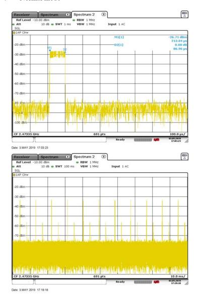
Time on of 100ms= 86.96us\*11=0.957ms Duty Cycle=0.957ms / 100ms= 0.00957 Duty Cycle correction factor= 20 LOG 0.00957= -40.386 dB
