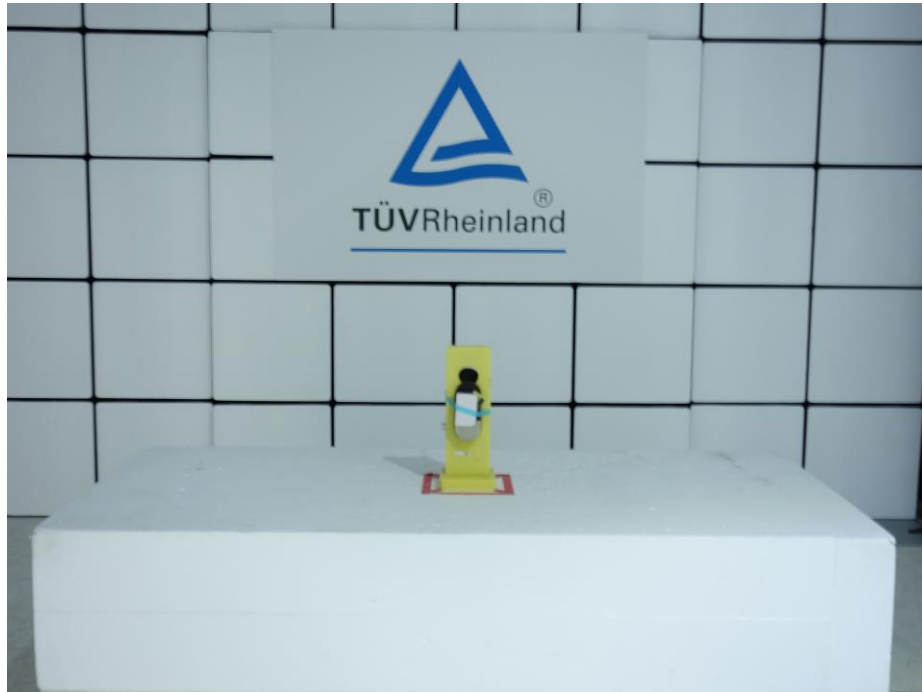
Photograph 1: Set-up for Spurious Emissions (Front View)
