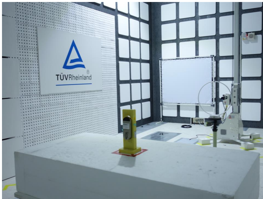
Photograph 2: Set-up for Spurious Emissions (Back View 1)
