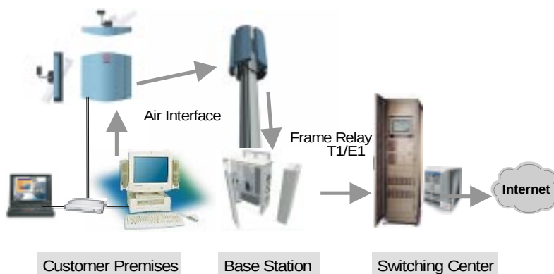
Figure 1-3 High Level System Architecture
