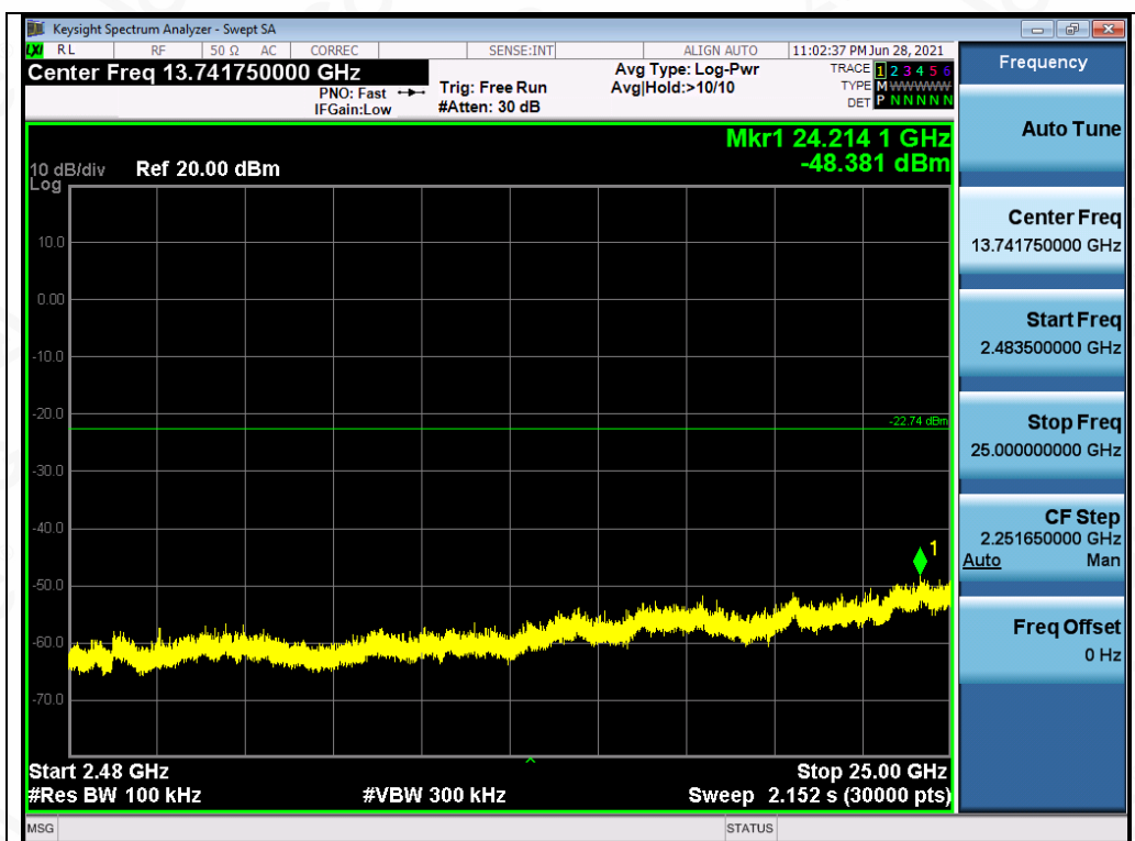
Test_Graph_BR_ANT1_2402_1Mbps_Higher Band Emissions
