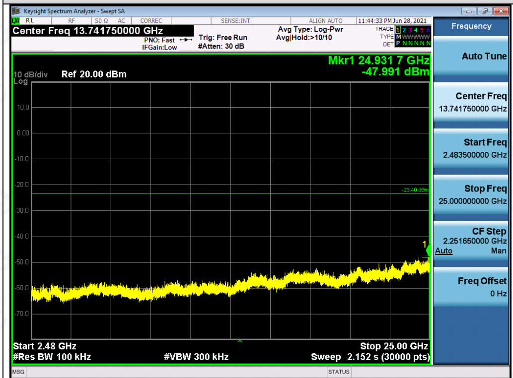
Test_Graph_EDR_ANT1_2441_3Mbps_Higher Band Emissions
