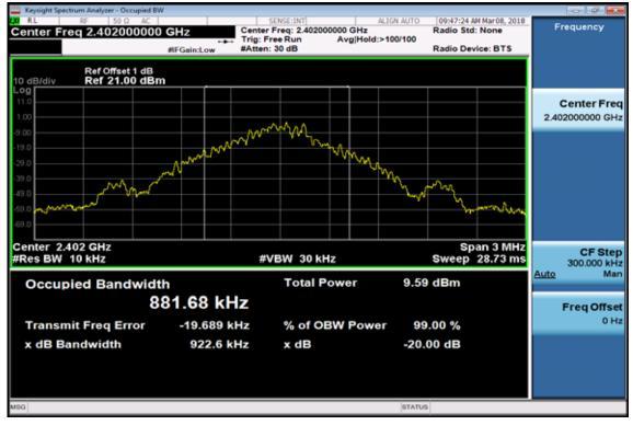
20dB Bandwidth Test Data CH-Mid
