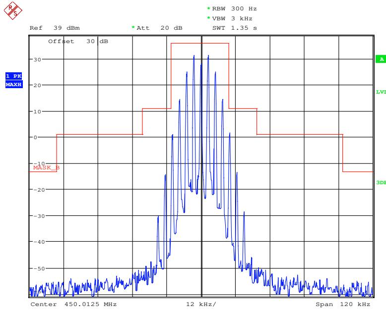
**Frequency 450.0125 MHz: Emission Mask B, Low Power, FCC part 74.462**
