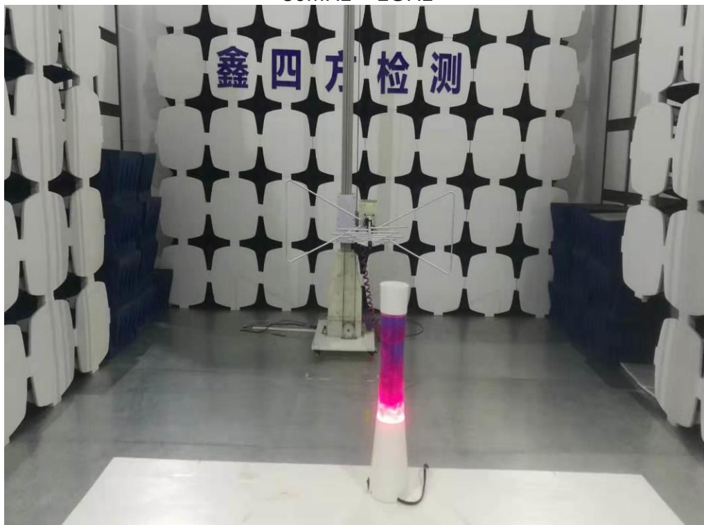
Photos of radiated emission test 30MHz – 1GHz
