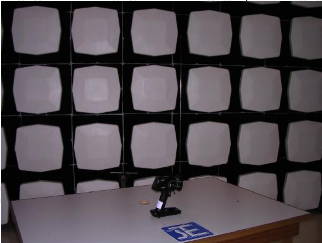
Measurement of Radiated Emission Test Set Up
