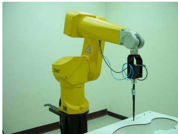
Fig. 5.2 Probe setup on robot
