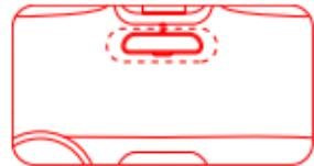
Note: Make sure to stick the electrostatic sticker on a flat and smooth part of the windshield, press it firmly, and avoid sticking it on the edge of the windshield's film to prevent it from falling down.
