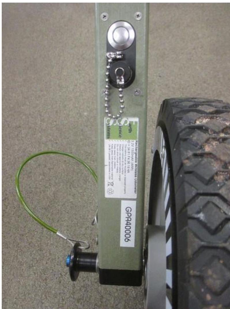
EUT Cart leg- Integrated wireless Odometer
