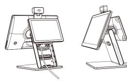
3. Align the top three clasps of the cover with the column clasps, and then press down the cover.
