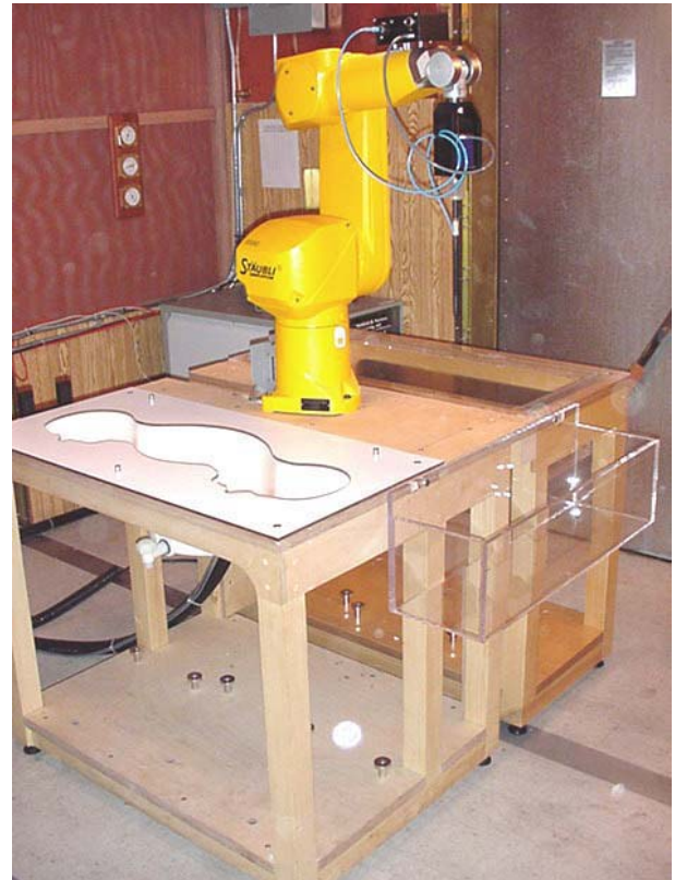
DASY4 SAR Measurement System with side-mount planar phantom
