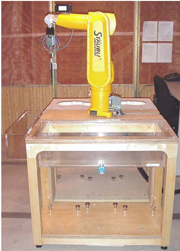
DASY4 SAR Measurement System with validation phantom
