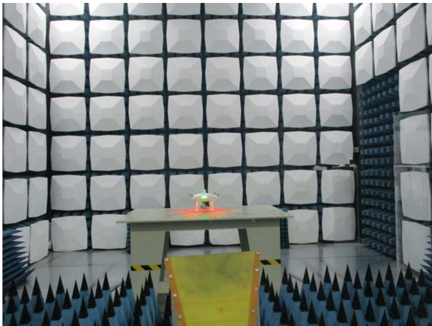
Radiated Emission Above 1GHz Rear View (Operating Mode)
