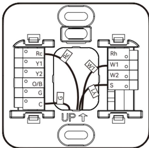
Tug on the wires gently to ensure they are secured. After all the wires are inserted, tuck them neatly back into the wall.
