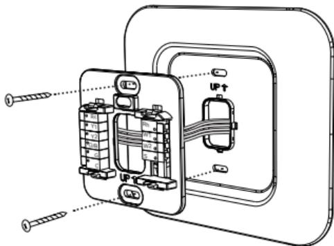
Optional: use the trim plate to cover screw holes or gaps left over from your old thermostat's installation.
