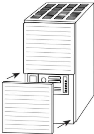
**Note:** Most HVAC systems have a safety switch will not start if the cover panel is not secure.
