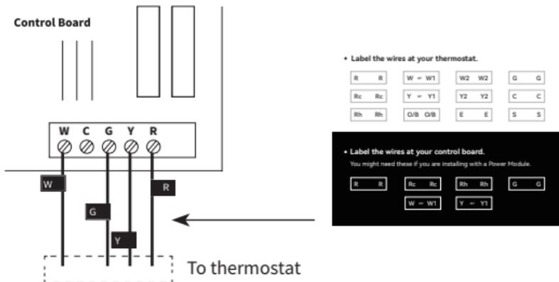
**Note:** If there are more than one wire connected to one terminal, only label the wire coming from the thermostat.
