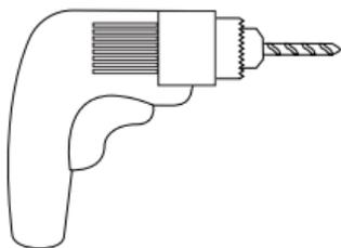
A drill with a 3/16-inch drill bit
