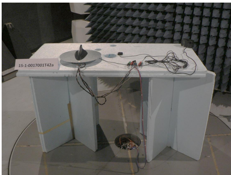
Photograph 3: Radiated measurements in semi-anechoic room (close view)
