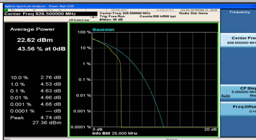
(Channel Bandwidth: 5 MHz)_LCH_QPSK_12RB#0
