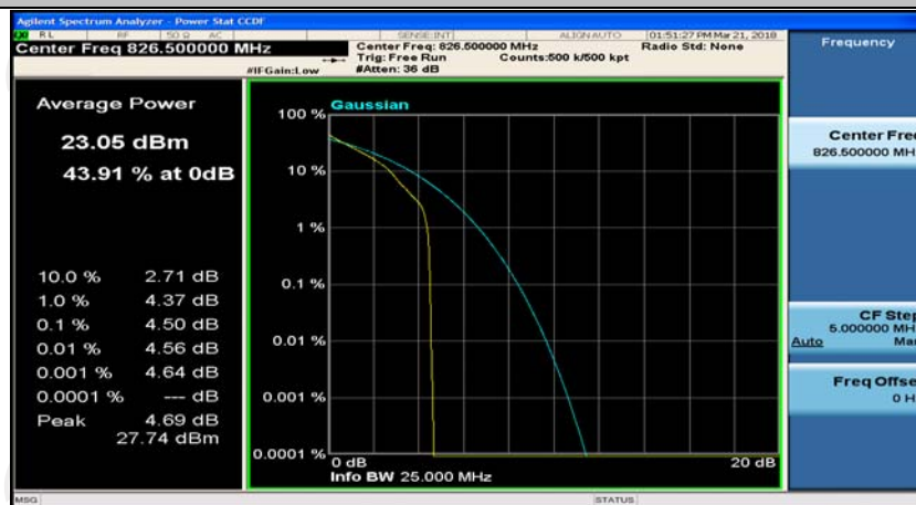
(Channel Bandwidth: 5 MHz)_LCH_QPSK_1RB#24
