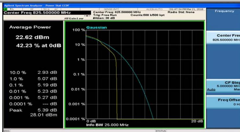
(Channel Bandwidth: 3 MHz)_LCH_16QAM_8RB#0
