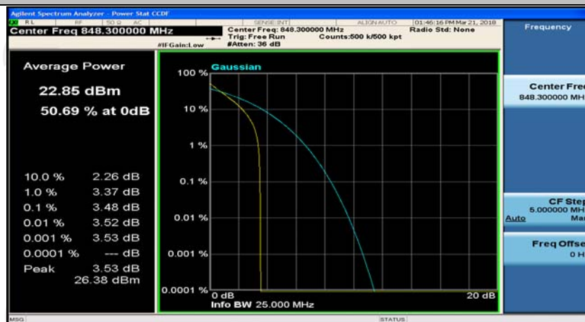
(Channel Bandwidth: 1.4 MHz)_HCH_QPSK_3RB#2
