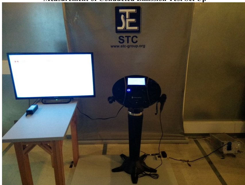
Measurement of Conducted Emission Test Set Up
