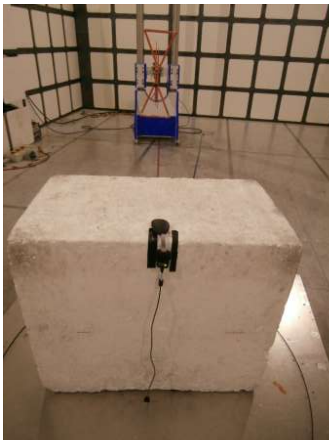
Figure 72 - Test Setup - 30 MHz to 1 GHz – X Orientation
