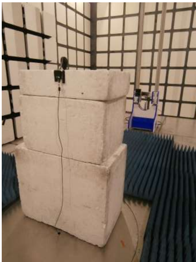
Figure 76 - Test Setup - 1 GHz to 18 GHz – Y Orientation
