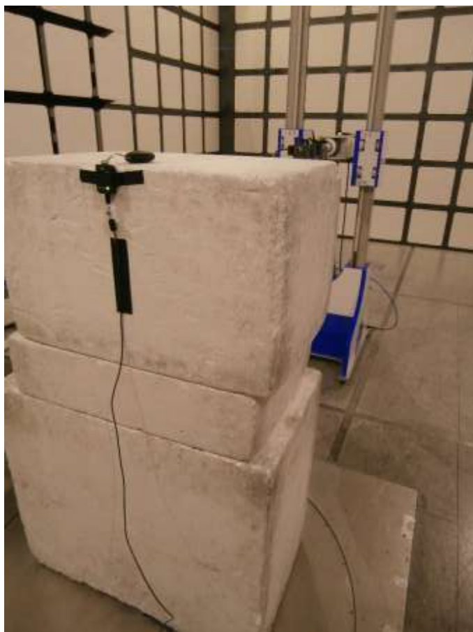
Figure 78 - Test Setup - 1 GHz to 25 GHz – X Orientation
