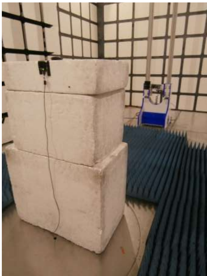
Figure 75 - Test Setup - 1 GHz to 18 GHz – X Orientation
