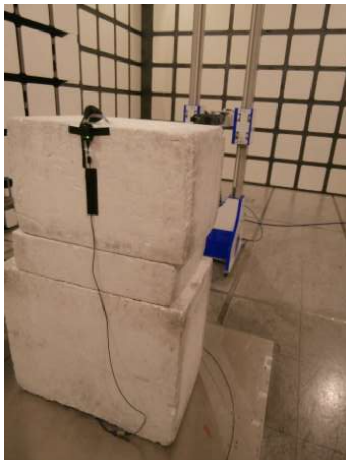
Figure 80 - Test Setup - 1 GHz to 25 GHz – Z Orientation
