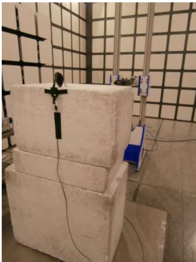
Figure 79 - Test Setup - 1 GHz to 25 GHz – Y Orientation
