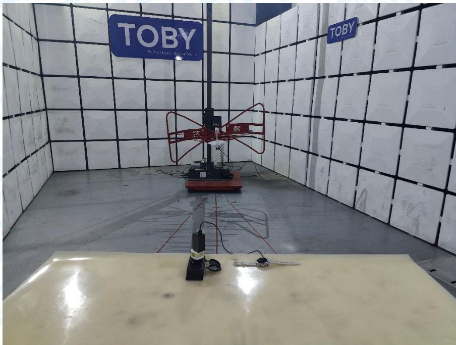
Photo of Setup for Radiated Emission (30MHz~1GHz)
