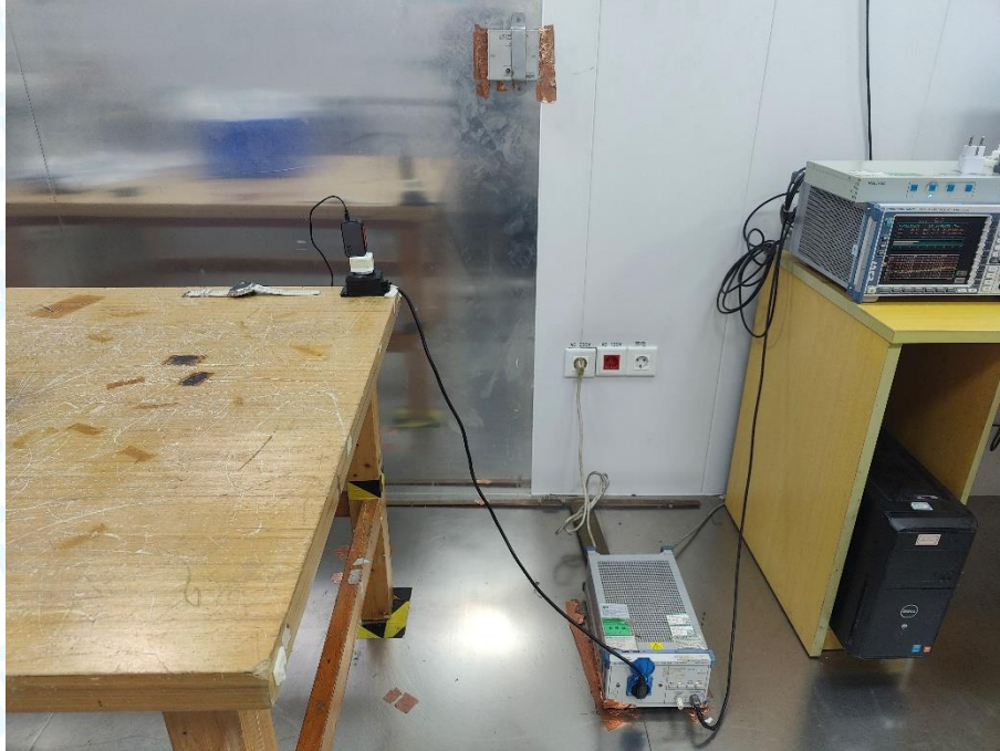
Photo of Setup for Radiated Emission (30MHz~1GHz)
