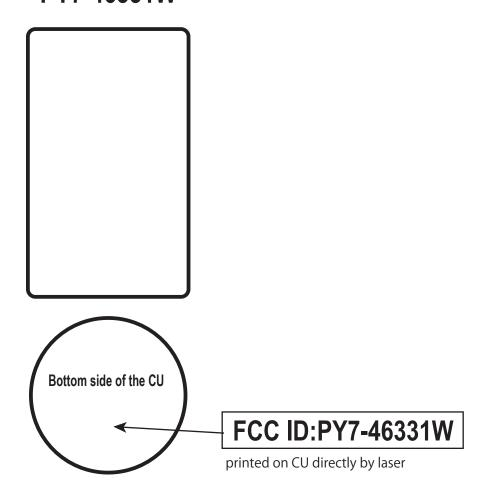
1. The FCC ID is on the label, FCC15.19(a) statement in manual due to device size
