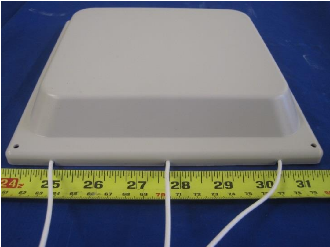
External Antenna- Front View
