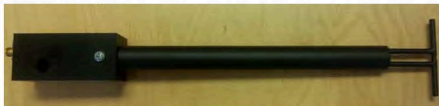
Figure 1 – MVG COMOSAR Validation Dipole
