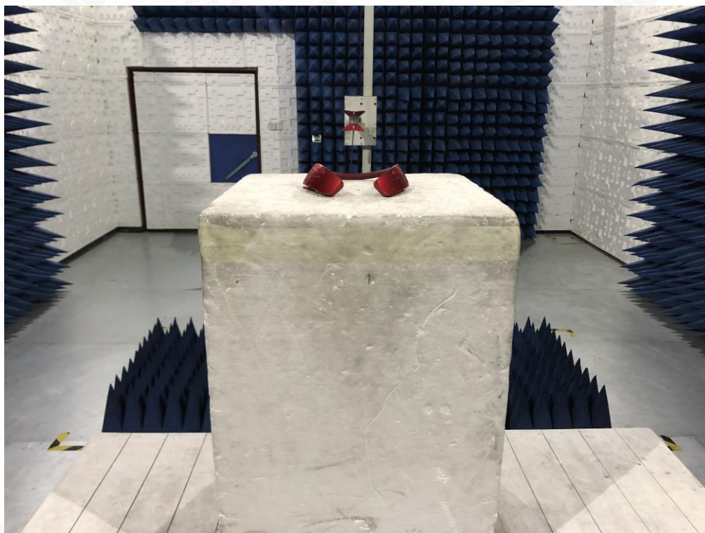
RADIATED EMISSION TEST SETUP ABOVE 1GHZ
