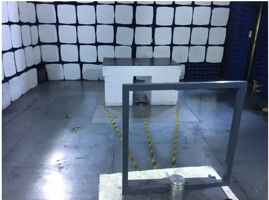
Radiation Emission Test Setup (Below 30MHz)
