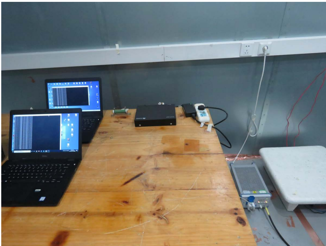
Picture 2 Conducted Emission Test Setup
