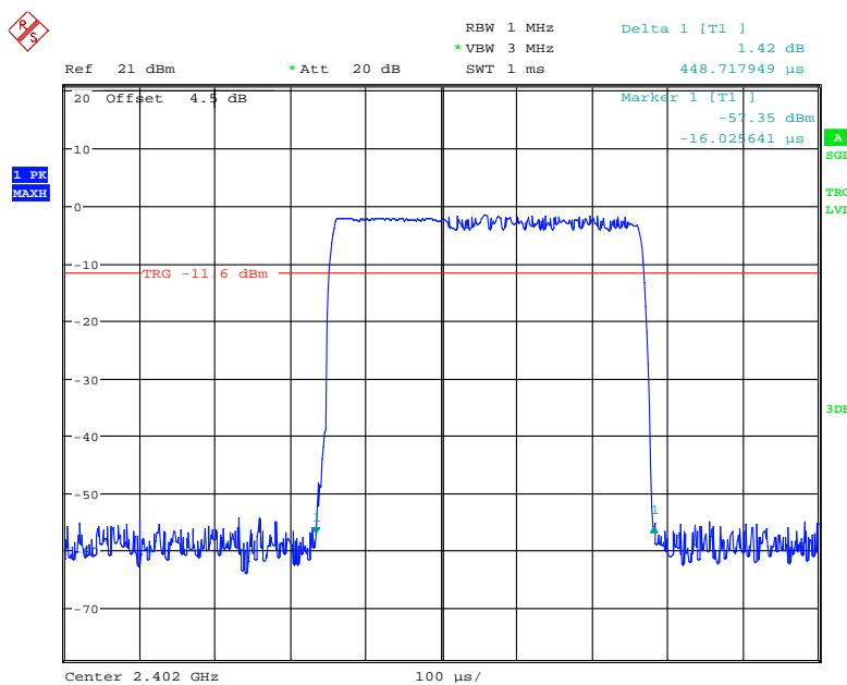
**Pulse time, Middle Channel, 2DH1**
