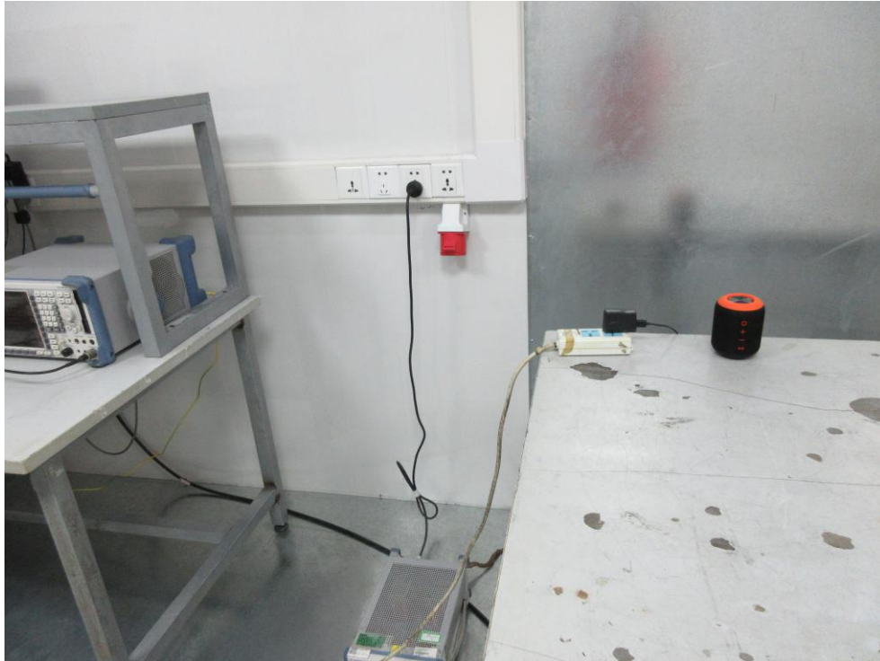
Photo of Conducted Emission Measurement
