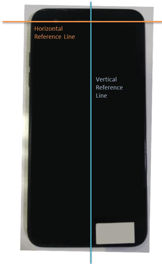
SAR Test Setup Photo 11: Horizontal and Vertical Reference Lines
