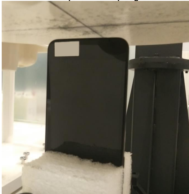
SAR Test Setup Photo 8: Bottom Edge at 1.0 cm
