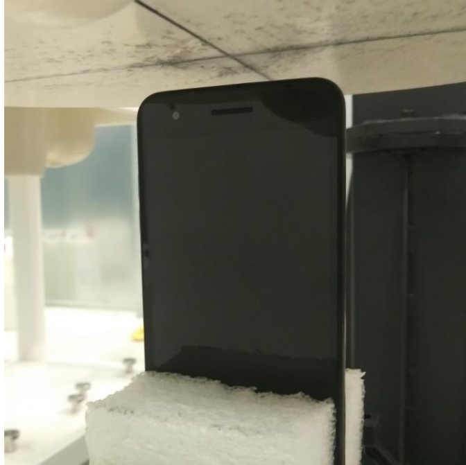
SAR Test Setup Photo 7: Top Edge at 1.0 cm
