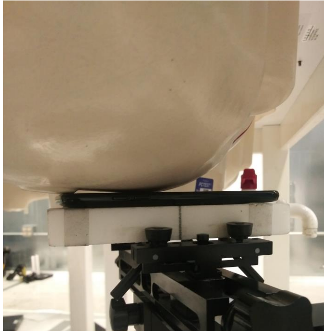
SAR Test Setup Photo 1: Right Cheek
