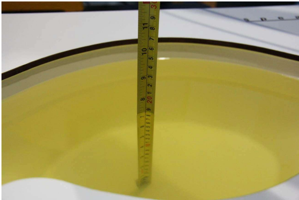
Picture 7-5: Liquid depth in the Flat Phantom(2450MHz)
