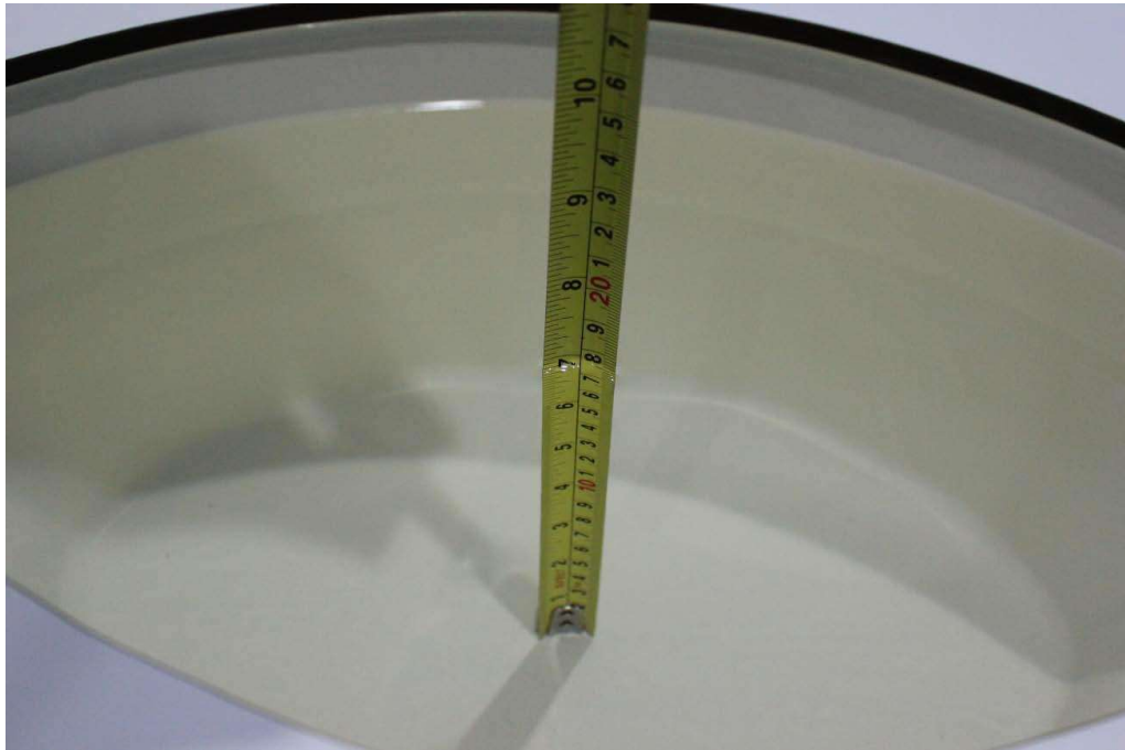
Picture 7-7: Liquid depth in the Flat Phantom(5GHz)
