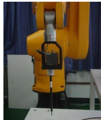
Picture C.3 E-field Probe
