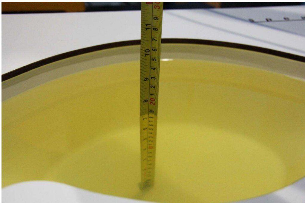
Picture 7-6: Liquid depth in the Flat Phantom(2550MHz)
