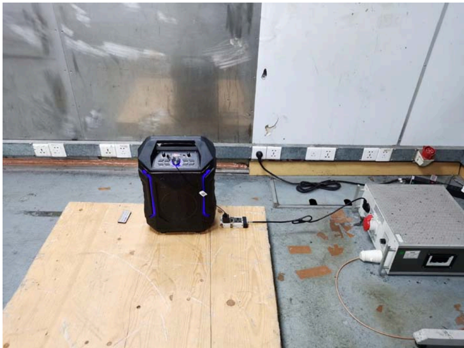
Photograph of set-up for AC mains Ports Conducted Emission
