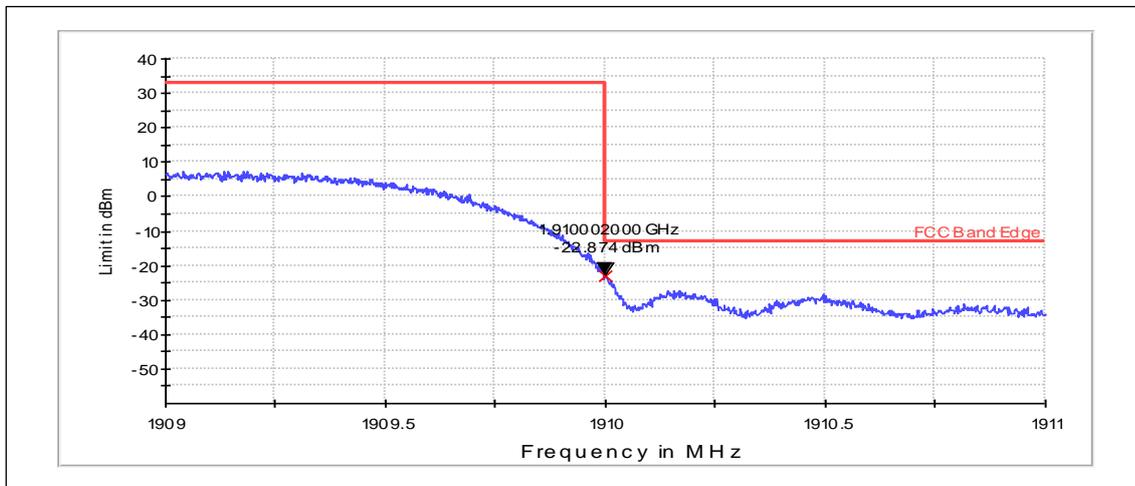
RMS (RBW: 50 kHz, VBW: 50 kHz, Max hold)
