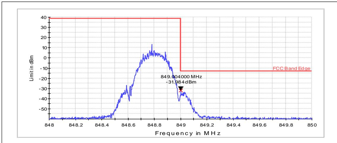
RMS (RBW: 3 kHz, VBW: 3 kHz, Max hold)
