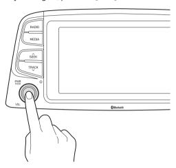
The system turns off when you stop the engine (ACC Off).
