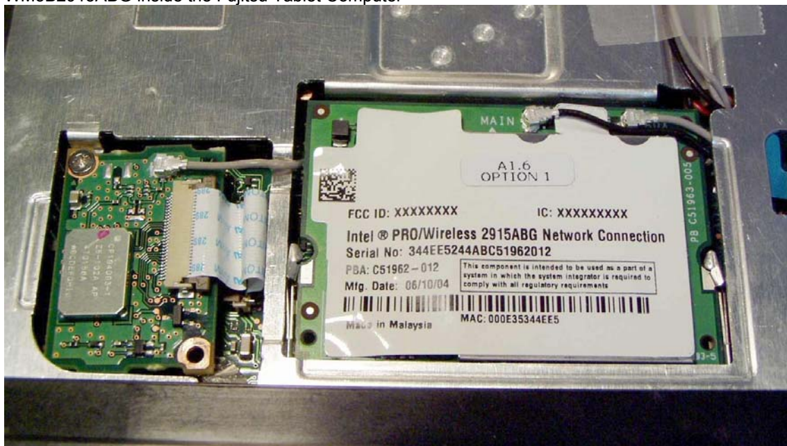
WM3B2915ABG inside the Fujitsu Tablet Computer
