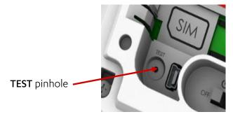
The C8000 LEDs flash and the C8000 beeps three times. The C8000 is restored to factory settings.
