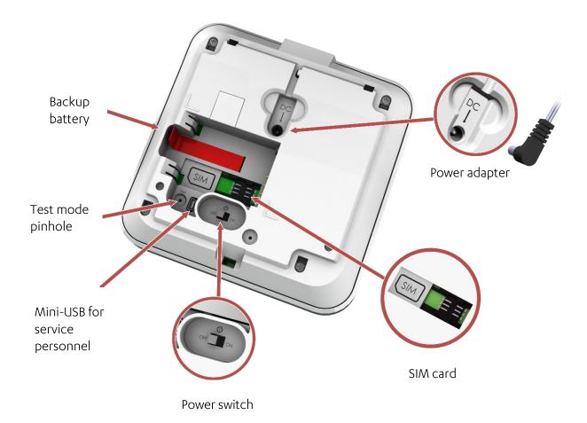
The C8000 has a rechargeable battery as a backup power source. The C8000 communicates with the monitoring station using a cellular network. If there is a communications failure, the C8000 saves messages and sends them when communication is restored.
