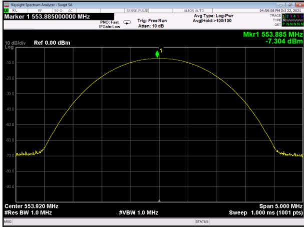
Test Plot-The Peak figure with modulation
