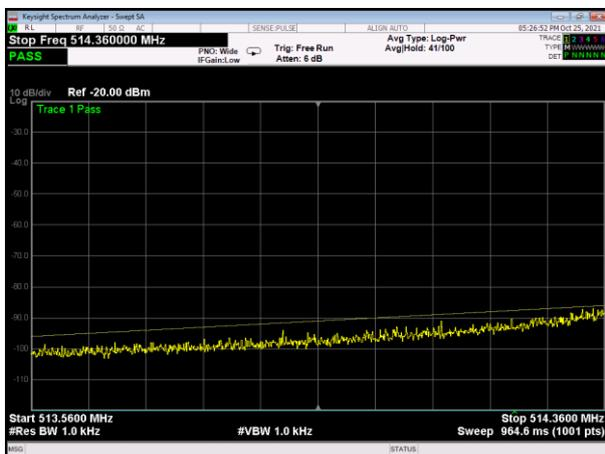
The Average figure with modulation (fc+B ~ fc+1MHz)
