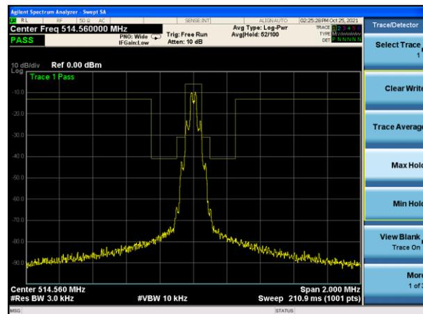
Test plot for M TX - 1 kHz
