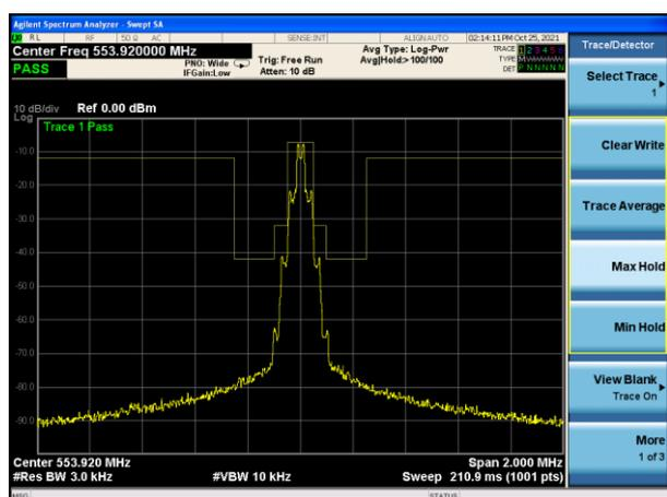
Test plot for H TX - 2.5 kHz
