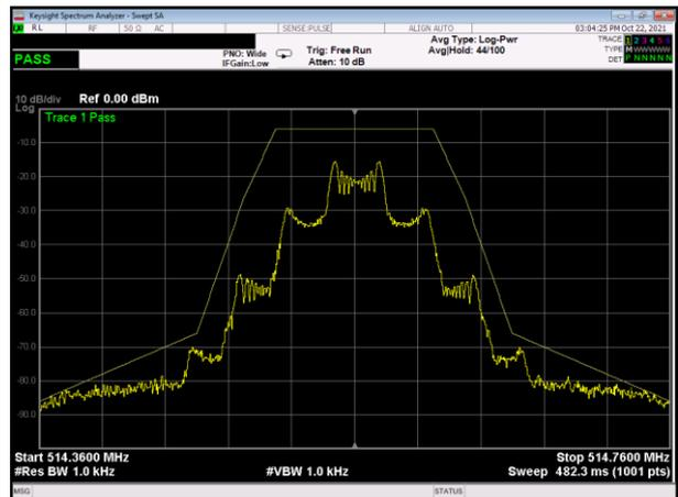
The Average figure with modulation (fc-1MHz~fc-B)
