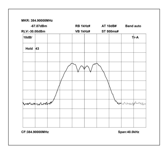
384.9MHz Signal Generator deviation set to 5kHz
