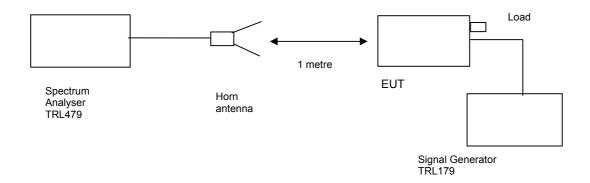
The test was set up as per the diagram. The level at the input was adjusted to compensate for the loss of the interconnecting cable. The unit was tested operating maximum power on three test frequencies with a 50 ohm load on the output. The unit was also tested with the signal generator replaced by another 50ohm load.
