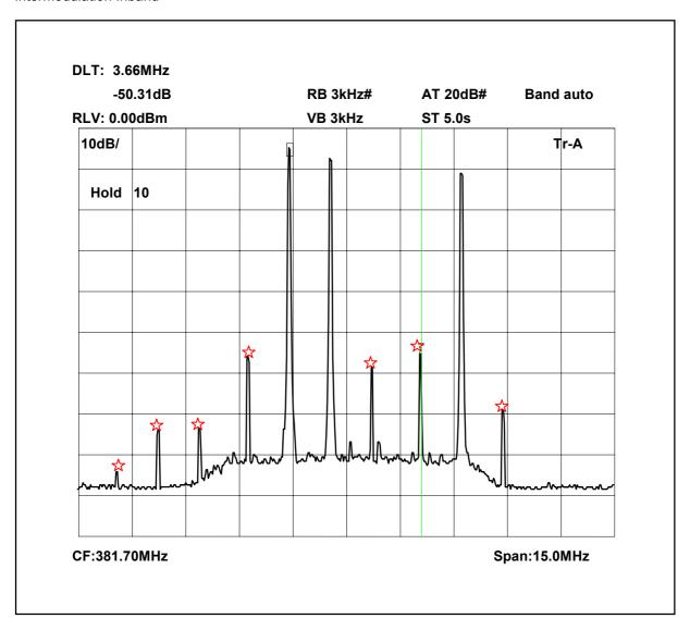
The above plot shows that all products (designated by  $\stackrel{\bigstar}{\sim}$ ) are at least 50dB below the fundamentals level detailed on previous page .
