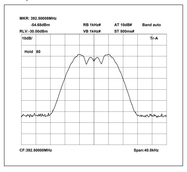
392.5MHz Signal Generator and amplifier deviation set to 5kHz
