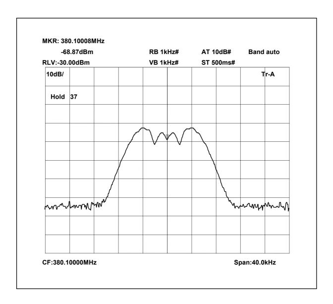
380.1MHz Signal Generator and EUT deviation set to 5kHz
