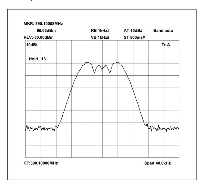
390.1MHz Signal Generator and EUT deviation set to 5kHz
